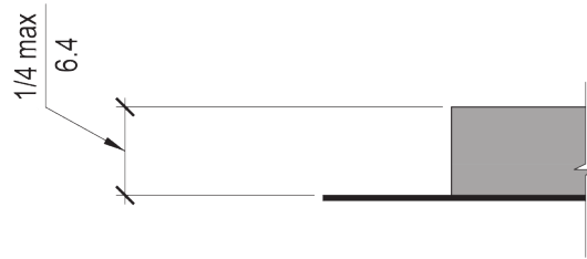
Fig.303.2 Vertical Changes in Level
