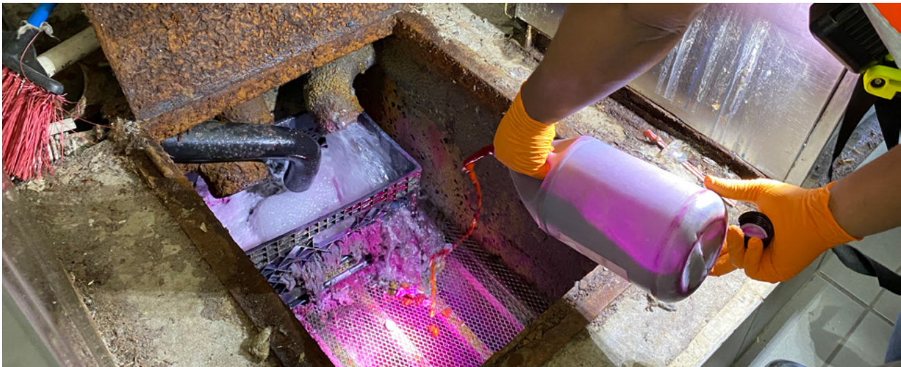
DEP conducts dye test to track down illicit discharge
