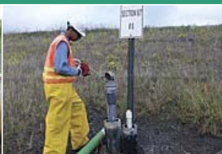
WORKER CHECKING LIQUID LEVEL IN CONDENSATE TANK
