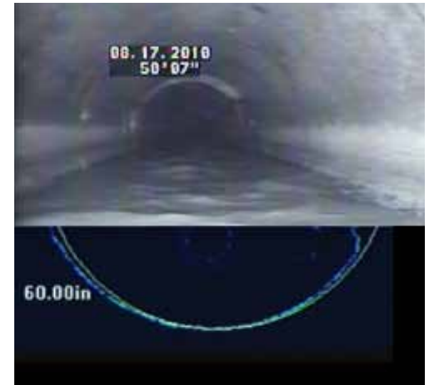
In both the above and below images, the top half shows a CCTV camera view of the sewer and the bottom shows the corresponding SONAR view below the water’s surface. Together these two technologies provide DEP with a comprehensive view of the sewer.
