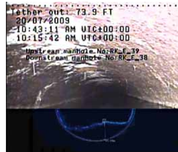
In both the above and below images, the top half shows a CCTV camera view of the sewer and the bottom shows the corresponding SONAR view below the water’s surface. Together these two technologies provide DEP with a comprehensive view of the sewer.
