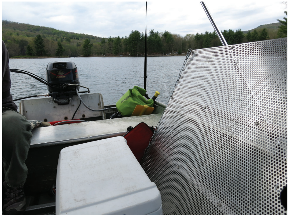
Figure 6. Bar check plate used during surveys of the West of Hudson reservoirs in New York State.
