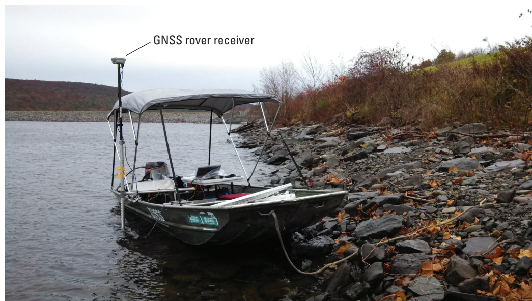
Figure 4. Survey boat and global navigation satellite system (GNSS) rover receiver used for the study of the West of Hudson reservoirs in New York State.
