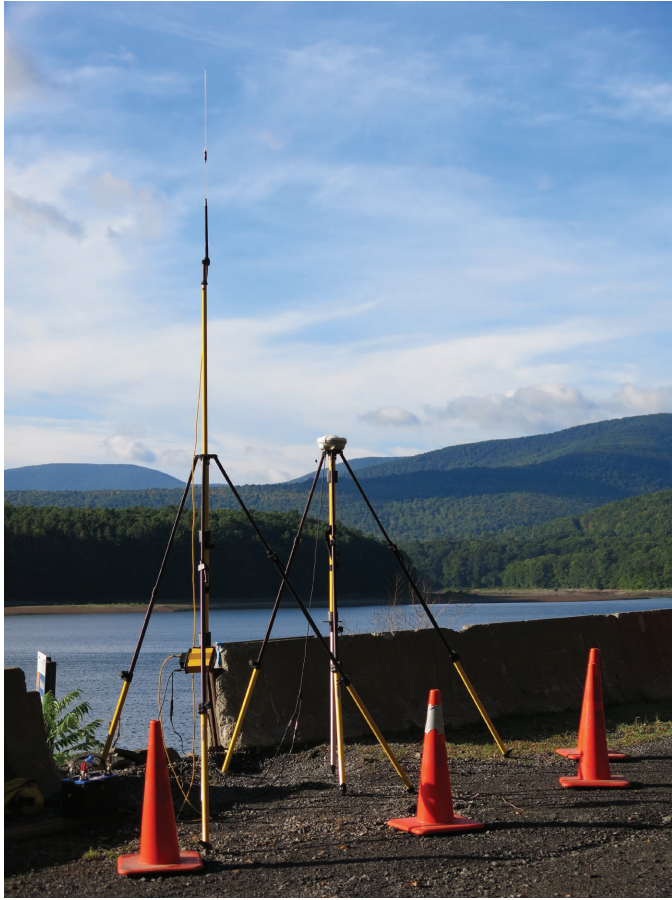
Figure 3. Base station and radio antenna at control point near Schoharie Reservoir, New York State.
