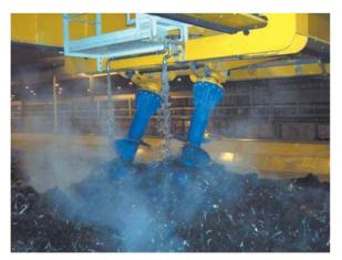
Photo 3-17: A system to add moisture to the composting material on the Edmonton facility air floor At any time during the air-floor–composting process, facility operators can add moisture to the material.
