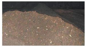
**Photo 1-12: Two-inch trommel screen "unders"** The two-inch unders, consisting primarily of immature compost, as well as smaller, non-degradable items, get transported to the air floor for further composting.
