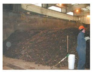
Photo 1-15: Removing samples from the windrows for laboratory analysis The Department took laboratory samples at different points during the 21 days that the NYC material spent on the Marlborough aeration floor.
