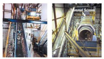
Photo 3-6: Conveyor belt (left) moving material to the Conporec primary trommel screen (right)
