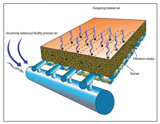
undesirable odors as by-products, including the rotten-egg smell of hydrogen sulfide gas. An adequate flow of air through the digesters, as well as during the first- and second-phase, post-drum composting processes, helps ensure that the recycling of the organic fraction of the waste stream will not generate undesirable odors within a pilot facility.
