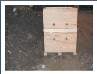
Photo 1-16: Cubic-yard sample shipped to lab for additional curing and testing The sample cured at the lab for an additional 21 weeks. At different points during this period, lab staff removed samples for analysis.
