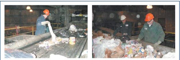
**Photo 1-7: Sort line at Marlborough facility** Following standard operations, workers at the Marlborough facility removed non-degradable items on the sort line before the NYC waste entered the composting drum.
