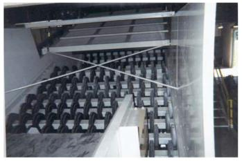
Photo 5-2: Debris Roll Screen at a Mixed-Waste MRF in Oakland, CA. Debris roll screens could be used in a pilot NYC facility to remove any small pieces of glass or plastic that were missed by the first screen.
