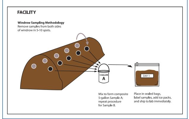
After all five days' worth of New York City's material was discharged from the drum, the unders covered one whole set of trenches and the windrow was complete (Illustration 1-3). At this point the Department took the next set of samples, which are labeled "Day 1" (see Illustration 1-4) on the laboratory data sheets attached as Appendix F.<sup>6</sup>
