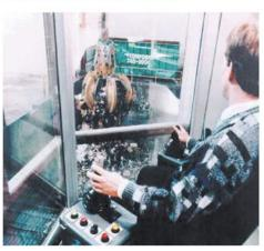
Photo 3-4: Conporec grapple crane operator From the control room, an operator uses a grapple to move waste from the pit to the bioreactor (composting) drum.
