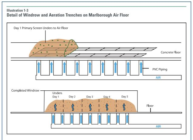
periodic turning (the strategy employed at Marlborough), or **aerated agitated bays**. In either case, active composting occurs inside a building with a system in place to capture and treat process air through a biofilter in order to minimize odors.
