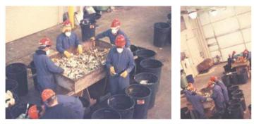
Photo 1-3: Sorting and characterizing samples of New York City waste Workers sorted samples of waste into 13 categories.
