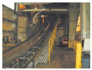
Photo 1-10: Conveyor belt leading to the two-inch, primary trommel screen
