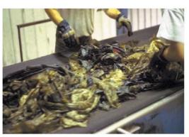
Photo 3-7: Removing recyclables from one-inch overs
