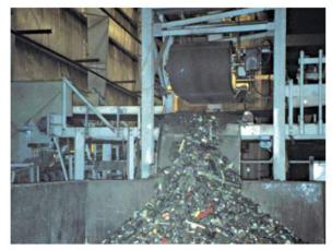
Photo 3-14: Conveyor to primary trommel screens (left) in the Edmonton facility and recovery of ferrous metals (right) Material discharged from the drum travels via conveyor to one of two three-inch trommel screens, which separates two fractions—"overs" and "unders." Before the three-inch unders move to the aeration bays, a magnet removes ferrous metals for recycling.
