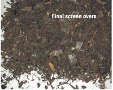
Photo 1-18: Samples of the NYC material passing under (top) and over (bottom) the three-eighths-inch screen Laboratory analysis confirmed Marlborough facility operators' criticism of the final screening equipment: 64.5% of the material passing over the final screen was compost.
