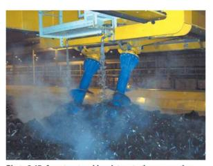
Photo 3-17: A system to add moisture to the composting material on the Edmonton facility air floor
