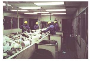
Photo 5-1: Example of an enclosed, climate-controlled sorting station
