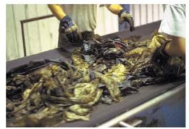
Photo 3-7: Removing recyclables from one-inch
