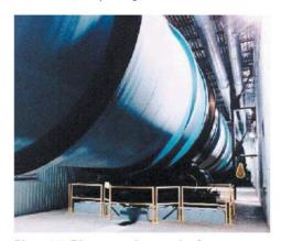
Photo 3-5: Bioreactor drum at the Conporec MSW-composting facility
