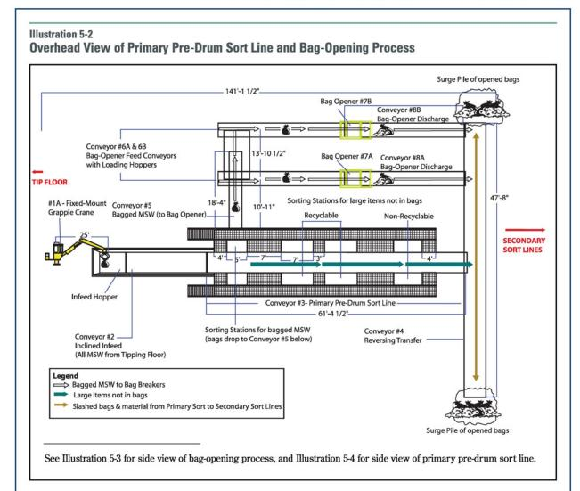
large conveyor (Conveyor #3). Conveyor #5 feeds into two conveyor lines (Conveyor #6A & 6B in Illustrations 5-2 and 5-3), which lead to **bag openers** (#7A & 7B) that slash open all of the
