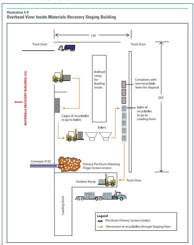
Depending on the amount and composition, the final debris roll screen **unders** (Conveyor #17A & 17B, Illustration 5-8) would either be disposed as residue or sent to the Materials-Recovery Staging Area for processing with the unders from the first set of primary pre-drum vibrating finger screens (Illustration 5-9).
