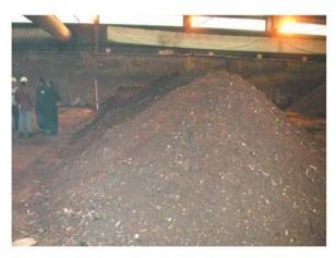
Photo 1-14: Windrow pile at the Marlborough facility Forming windrows on aerated floors represents one of the ways that MSW-composting facilities maximize decomposition rates and minimize odors.
