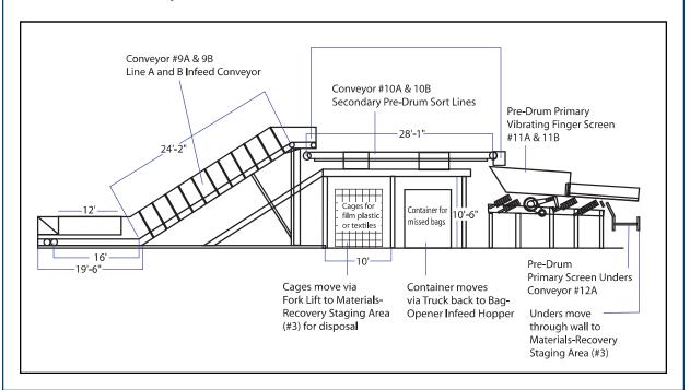
Side View of Movement of Pre-Drum Primary Screen Unders
