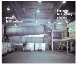
Photo 3-24: Sorting system at the Rapid City MRF The recycling-sorting system consists of two, enclosed sorting stations with space for six or more pickers, an air classifier (for plastic), a magnet (for ferrous), and an eddy current separator (for aluminum).
