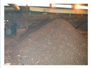
**Photo 1-14: Windrow pile at the Marlborough facility** Forming windrows on aerated floors represents one of the ways that MSW-composting facilities maximize decomposition rates and minimize odors.
