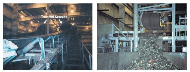
Photo 3-14: Conveyor to primary trommel screens (left) in the Edmonton facility and recovery of ferrous metals (right) Material discharged from the drum travels via conveyor to one of two three-inch trommel screens, which separates two fractions—"overs" and "unders." Before the three-inch unders move to the aeration bays, a magnet removes ferrous metals for recycling.
