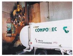
Photo 3-3: Inside the Conporec tipping building After crossing the weigh scale, trucks empty solid waste into a large waste pit.
