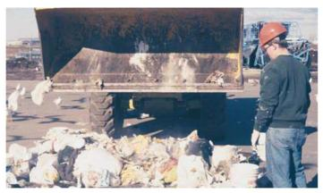
Photo 1-2: Removing samples for waste characterization Under supervision of the sampling coordinator, a front-end loader removed one to two samples from each pile.
