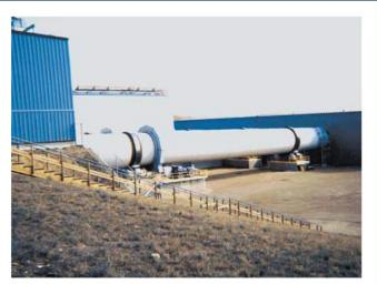
Photo 3-13: Digester drums at Edmonton facility Edmonton employs five digester drums, each measuring 16 feet in diameter and 242 feet in length.
