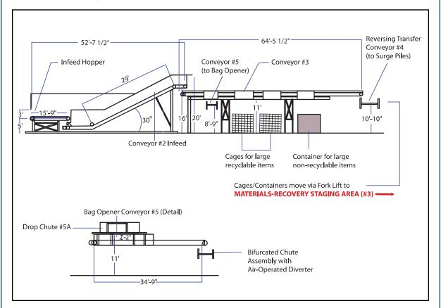
Illustration 5-5 Overhead View of Secondary Pre-Drum Sort Lines
