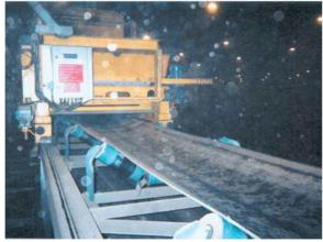
Photo 3-15: Edmonton aeration hall (before facility operation) and closeup of the conveyor and sidecar system Edmonton employs a mechanized approach to the air-floor composting process. Conveyors and sidecars (above right) automatically load the bays with immature compost. Three separate bridge cranes (like the one shown above left) straddle each bay and move up and down its length.
