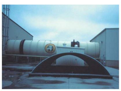
Photo 3-26: Digester drum at the Rapid City MSW-composting facility
