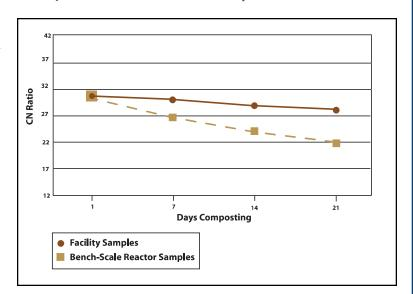
Figure 3-2 CN Changes During Composting of NYC Waste Streams: Facility vs. Bench-Scale Reactor Samples
