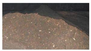
Photo 1-12: Two-inch trommel screen "unders"
