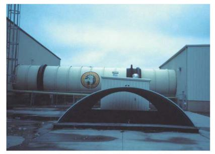
**Photo 3-26: Digester drum at the Rapid City MSW-composting facility** The facility uses two digester drums, each 14 feet in diameter and 79 feet long. The loading and discharge ends are enclosed inside two different buildings.
