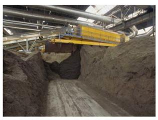
Photo 5-4: Finished compost after final facility screen
