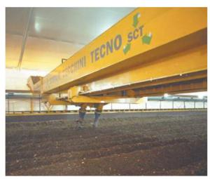
Photo 3-16: Close-up view of an auger mounted on a bridge crane in the Edmonton facility
