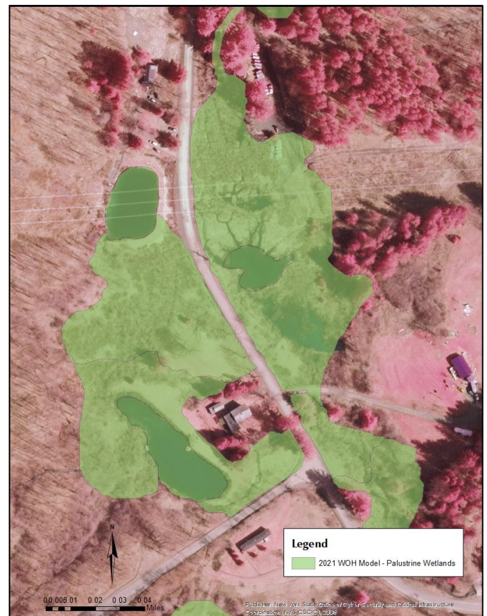
Figure 6. Road features were erased from this wetland polygon within the Cannonsville Basin using land use/land cover data.
