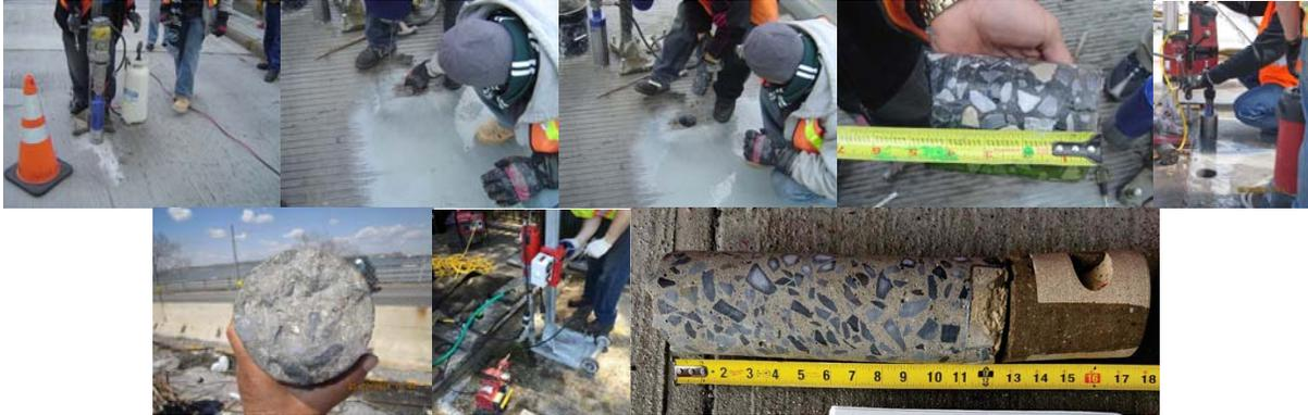
Removing a Core from 252<sup>nd</sup> Street Bridge over Henry Hudson Parkway in January 2009. (Credit: Masroor Mahmood) Core Sampling on the Bay Ridge Avenue Bridge in 2014. Utilizing a Coring Machine to Obtain a Concrete Core for Testing in June 2016 from the Westbound BOE over Adams Street.
