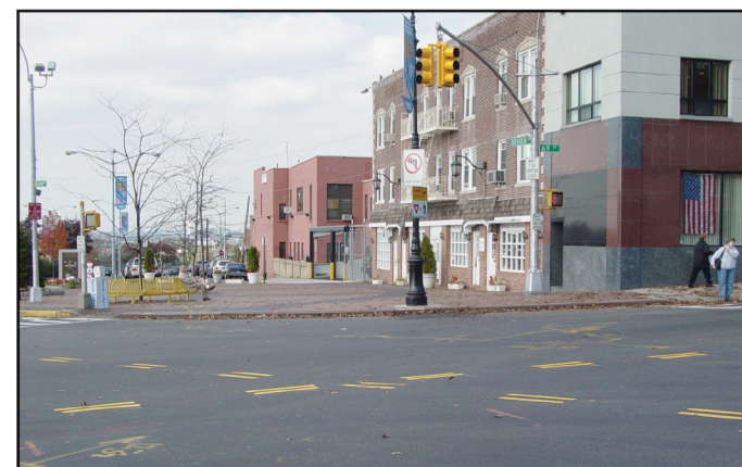
Above: Roadway markings including peg-a-tracs
