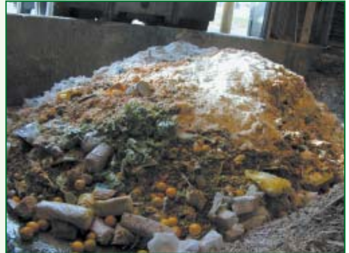
Food waste is comprised of pre-consumer waste as well as leftover prepared food and post-consumption plate scrapings. Facility operators mix this material with wood chips (shown below) before loading it into the concrete bays.
