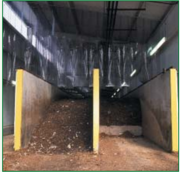
The agitator, pictured above, moves along the bays, slowly pushing the material forward as it mixes it. After 14 days in the bays, the food waste has broken down into compost.
