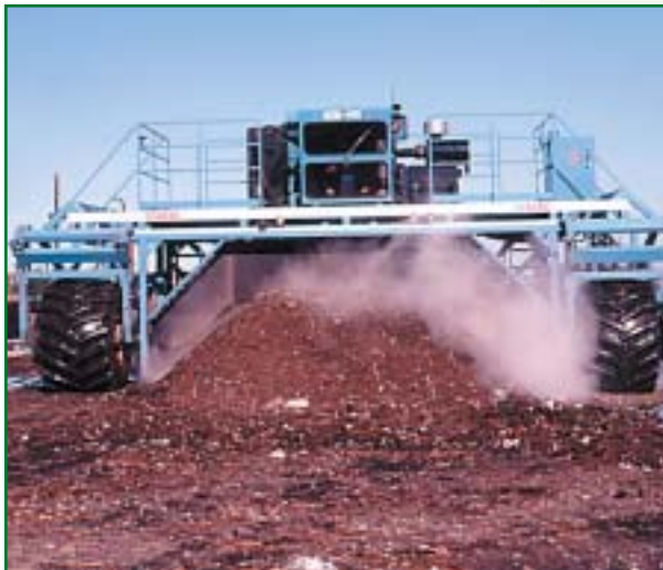
Turning the windrows at the Fresh Kills compost facility.
