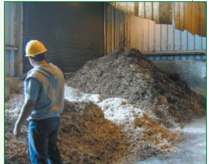
Food waste is comprised of pre-consumer waste as well as leftover prepared food and post-consumption plate scrapings. Facility operators mix this material with wood chips (shown below) before loading it into the concrete bays.
