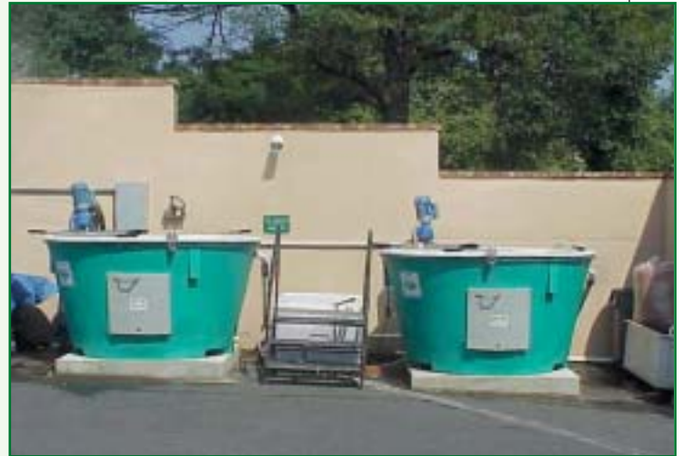
“Earth Tubs” are examples of small, in-vessel units the Department has helped to install at several City institutions to test the feasibility of on-site composting of food waste.
