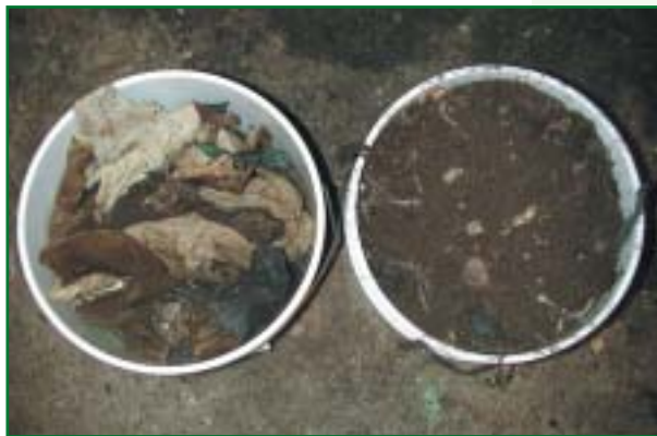
After three days in the drum, the organic fraction of the waste had broken down into an immature compost. The material then passed over a two-inch screen, where the large inorganic items that did not break down were pulled out for disposal. The bucket on the left contains a sample of the two-inch “overs” (the material that was rejected by the two-inch trommel screen) and the one on the right holds the two-inch “unders” (or immature compost). Note that much of what was pulled out was plastic bags.
