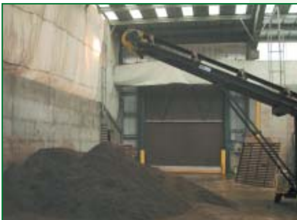
The NYC material was run through a final 3/8-inch screen to remove particles of glass, plastic, and other fine contaminants.
