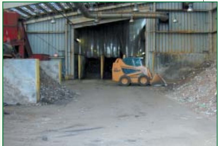
After operators remove compost from the back end of the bays, they form it into piles in the indoor curing area at the back of the facility.
