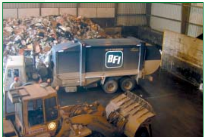
Incoming waste is unloaded onto a tipping floor at the Marlborough mixed-waste-composting facility. Bulky items, such as mattresses, are pushed aside with a front-end loader.
