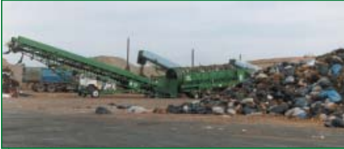
At compost sites, collected leaves are passed through a trommel screen to remove the plastic bags and reduce the size of the leaves.
