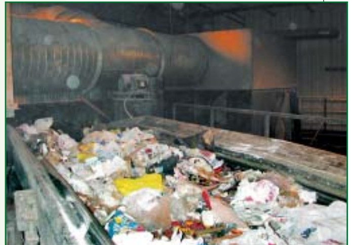
NYC waste enters the composting drum via a conveyor belt. A waste characterization showed that 55 percent of the material is biodegradable.
