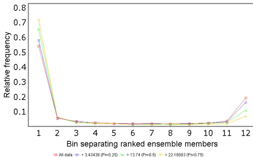
Figure 6.15. Verification rank histogram for ensemble of 11 GEFS forecasts of daily maximum temperature at lead hour 48 for Schoharie Reservoir site. The GEFS forecasts are for 1984-2018 and the corresponding observations are obtained from PRISM gridded data set.
