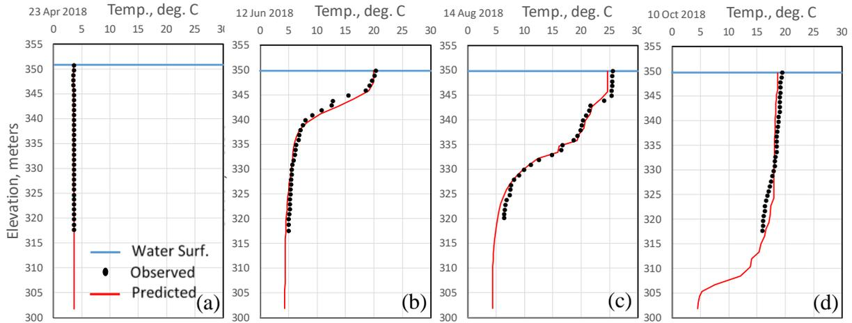
Figure 6.22 Observed and predicted water temperature ( $^{\circ}\text{C}$ ) in the water column of Cannonsville Reservoir, 2018: (a) April 23 (initial condition), (b) June 12, (c) August 14, and (d) October 10.
