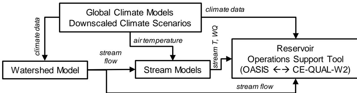
Figure 6.11. System of models for assessing impact of climate change on NYC's water supply system. Stream T, WQ refers to stream temperature and water quality; OASIS and CE-QUAL-W2 are reservoir operations and reservoir water quality models, respectively.
