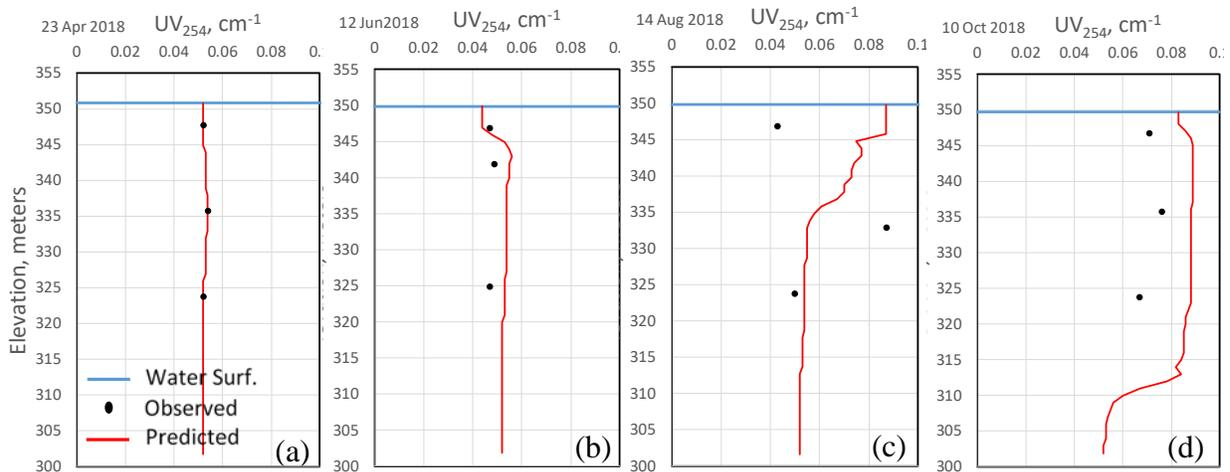
Figure 6.23 Observed and predicted  $UV_{254}$  ( $\text{cm}^{-1}$ ) in the water column of Cannonsville Reservoir, 2018: (a) April 23 (initial condition), (b) June 12, (c) August 14, and (d) October 10.
