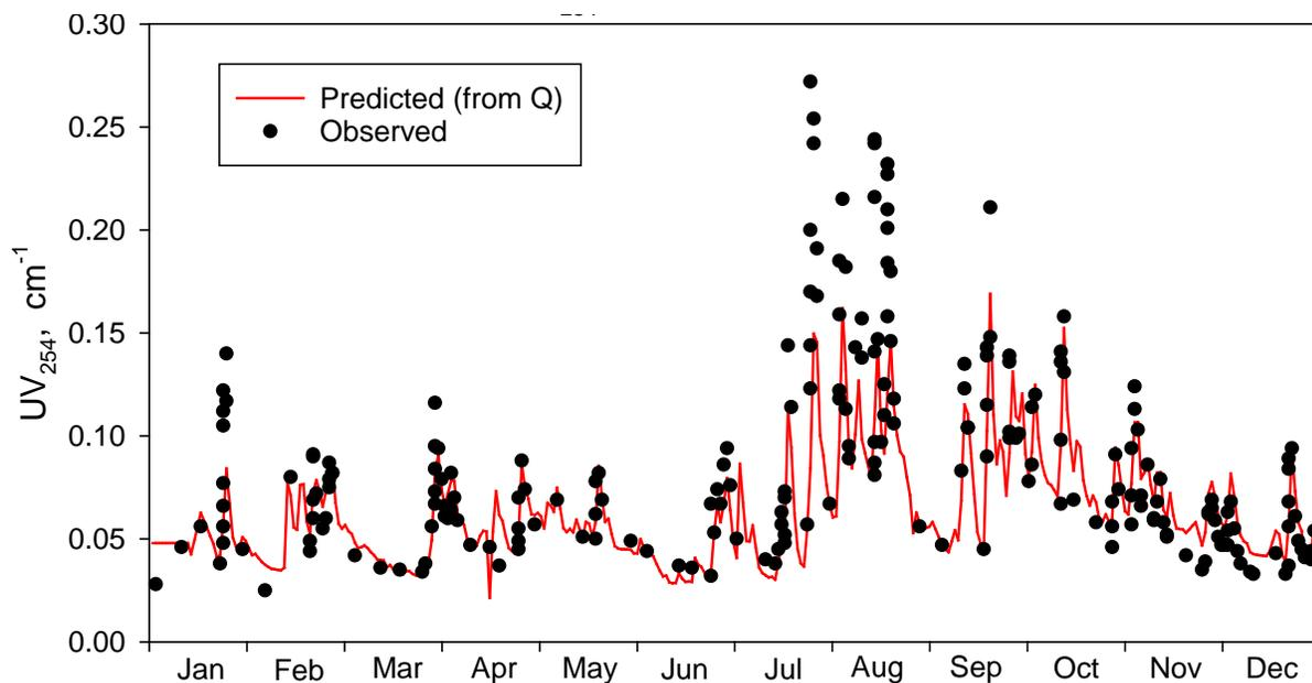
Figure 6.21 Observed and predicted  $UV_{254}$  levels for the West Branch Delaware River, 2018. Observations are the black circles ( $n=225$ ), while the predictions are daily values based on the measured USGS daily average streamflow measured at the Walton gage, and using Equation (6-2).
