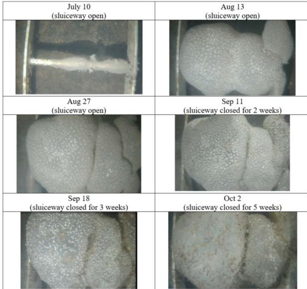
Figure 4.7 Late sluiceway closure - time-series photos from Shaft 18 sluiceway 2 showing the size and condition of *P. magnifica* from July 10 to October 2, 2019, with colony senescence visible at September 18, 2019. For scale, each of the ladder rungs is about 12 inches across.
