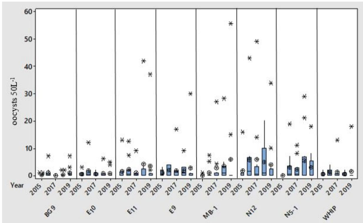
Figure 5.10 *Cryptosporidium* concentrations by year for routine samples at the eight Kensico streams from 2015 through 2019.
