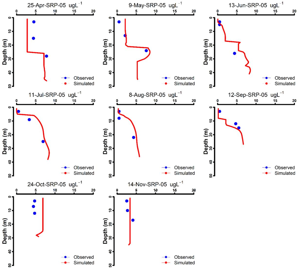
Figure 6.20. Predicted and observed vertical profiles of soluble reactive phosphorus (SRP) ( $\mu\text{gL}^{-1}$ ) in Cannonsville Reservoir, April through October 2005.
