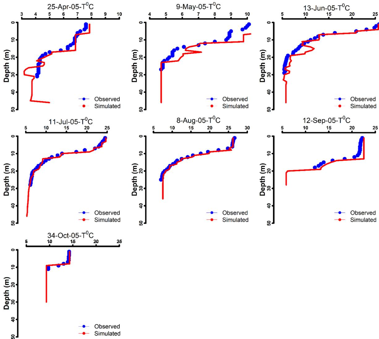
Figure 6.17. Predicted and observed vertical profiles of temperature ( $^{\circ}\text{C}$ ) in Cannonsville Reservoir, April through October 2005.
