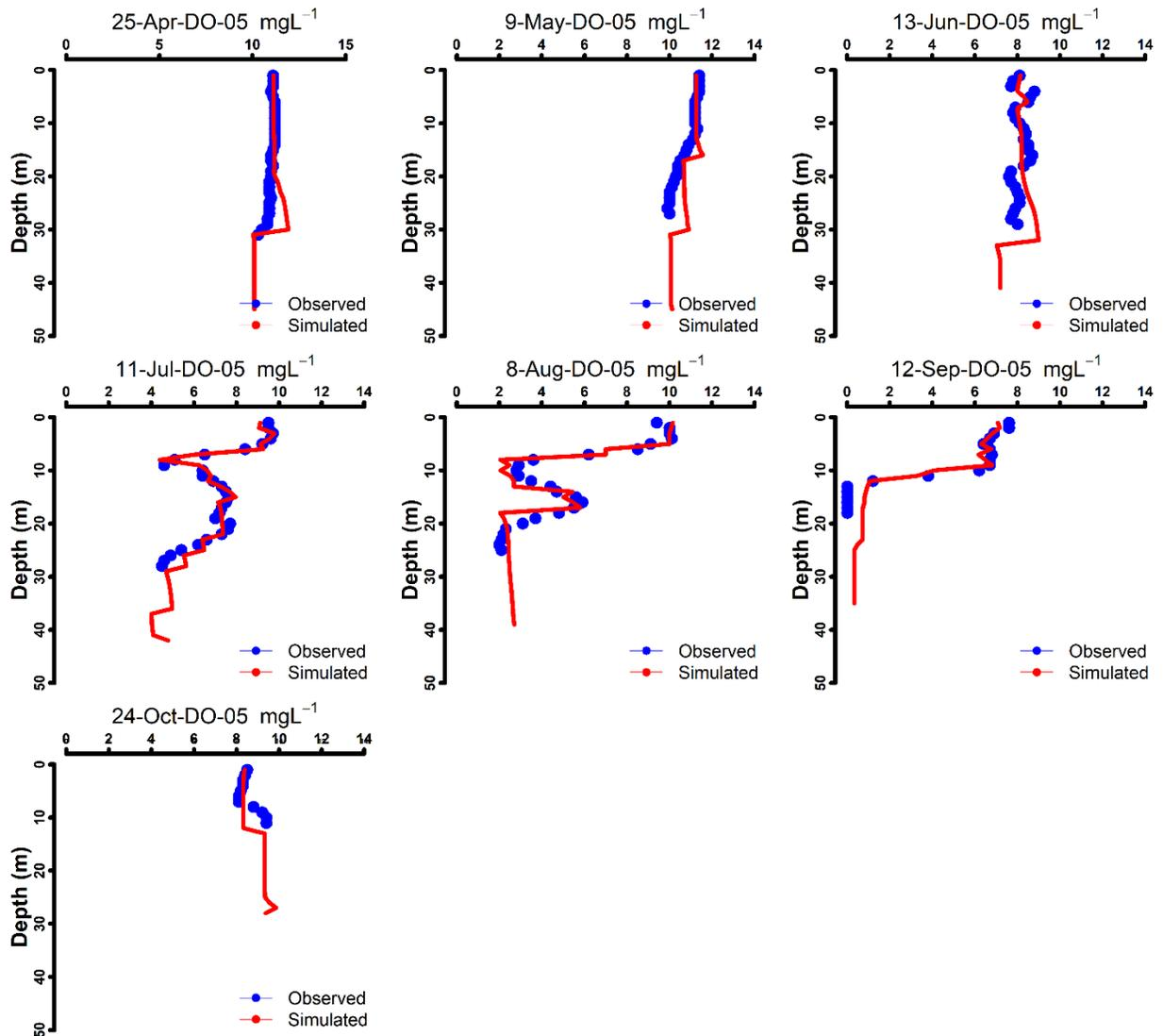
Figure 6.18 Predicted and observed vertical profiles of dissolved oxygen (DO) ( $\text{mgL}^{-1}$ ) in Cannonsville Reservoir, April through October 2005.
