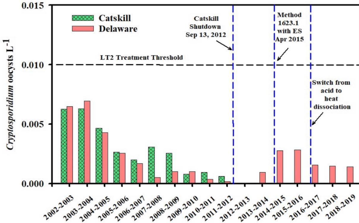
Figure 5.8 *Cryptosporidium* means using LT2 calculation method since initiation of Method 1623HV (1623.1 with EasyStain since April 2015) at the Delaware Aqueduct 2002-2018 and the Catskill Aqueduct 2002-2012.
