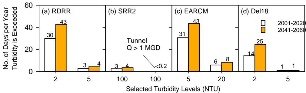
Figure 6.13 Predicted number of days per year when turbidity is exceeded by specific levels at (a) Rondout Reservoir diversion, RDRRCM, (b) Schoharie Reservoir diversion, SRR2CM, (c) Ashokan Reservoir diversion, EARCM, and (d) Kensico Reservoir diversion, DEL18DT, for the baseline (2001-2020) and future (2041-2060) climate scenarios (20 GCMs; RCP 8.5).
