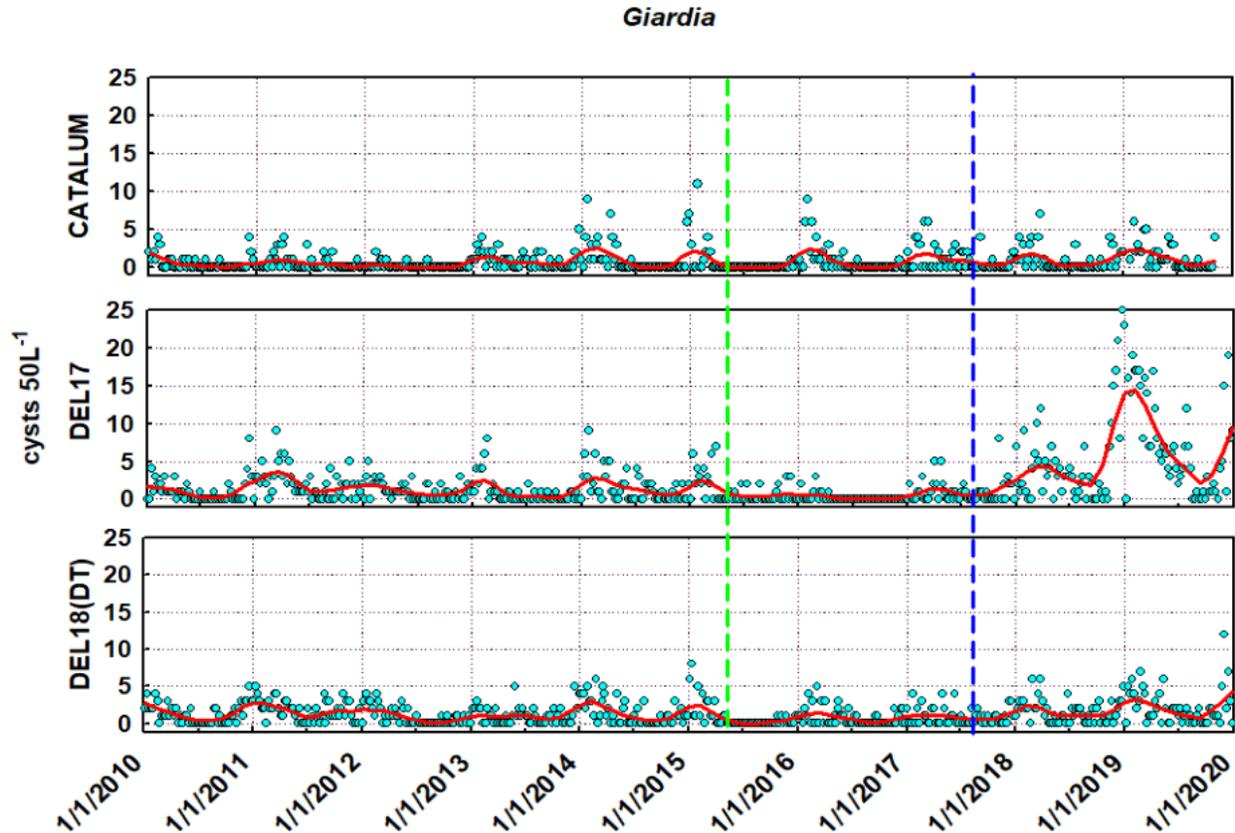
Figure 5.7 Weekly routine source water keypoint results for *Giardia* (circles), and LOWESS 5% smoothed regression (red curved line) from October 15, 2001 to December 31, 2019. The green dashed line indicates the change from Method 1623HV to Method 1623.1 with EasyStain. The blue dashed line indicates the laboratory method modification from acid to heat dissociation. \*The New Croton Reservoir outflow is no longer included in this analysis since results are only quarterly.
