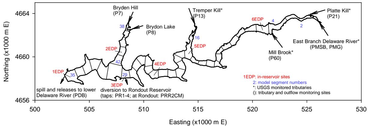
Figure 6.16 Pepacton Reservoir: Inflows, outflows, in-stream and in-reservoir routine water quality monitoring locations, and w2 model segments. Selected model segments are also numbered according to the numbering scheme of w2.
