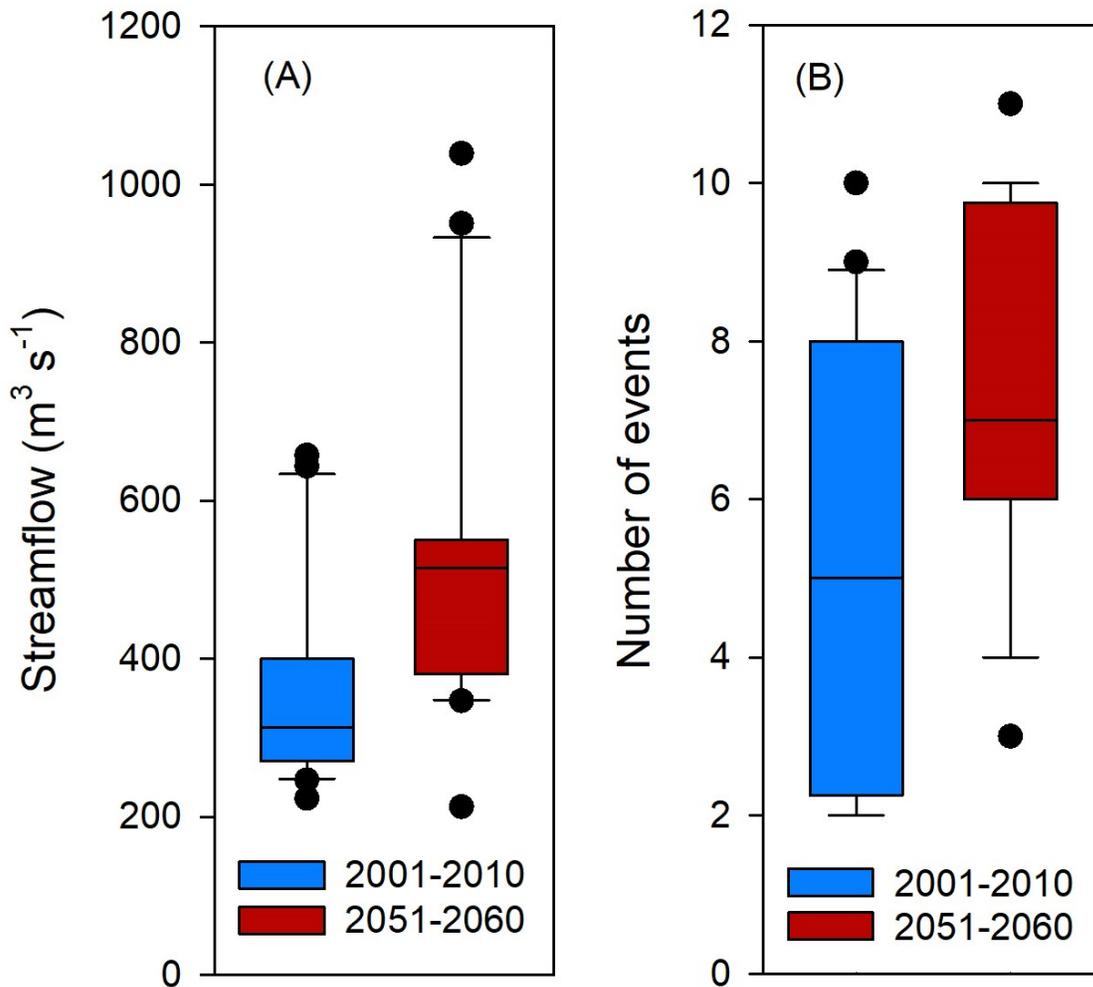
Figure 6.7. (a) Simulated magnitude of largest event in a 10-year period by each of the 20 GCM for the RCP 8.5 emission scenario (b) Projected change in frequency of events when streamflow exceeds  $200 \text{ m}^3 \text{ s}^{-1}$  at the West Branch Delaware River at Walton USGS flow station.
