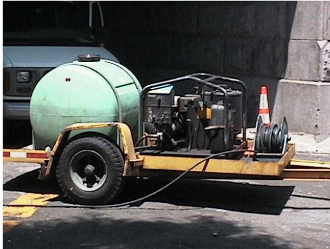
Pressure Washing Machine Used for Graffiti Removal.
