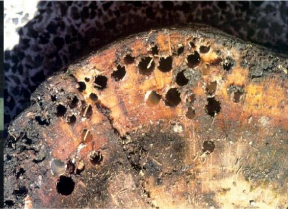
Teredo Damage (holes up to 1/4" diameter)
