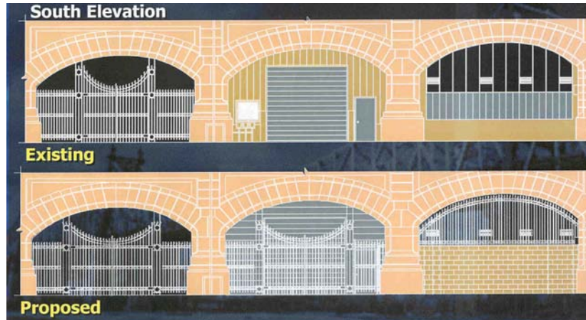
Proposed Rehabilitation of the Arch Infill for the Sanitation Department
