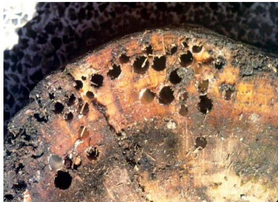
Teredo Damage (holes up to ¼" diameter)
