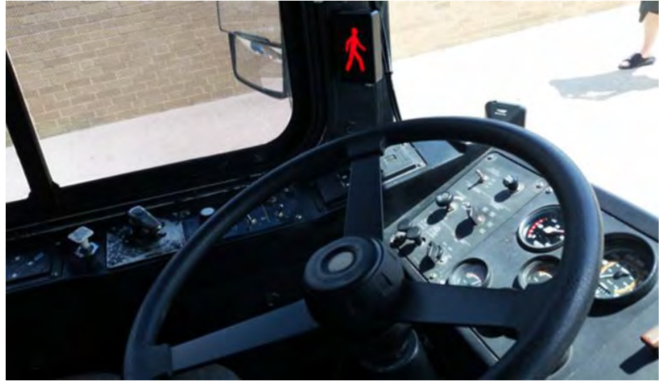
MTA Collision Avoidance System installed on a city bus.
