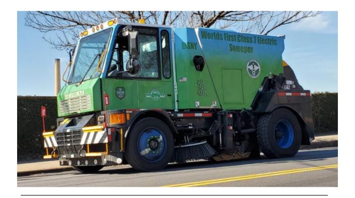
NYC's First Battery-Electric Mechanical Broom
