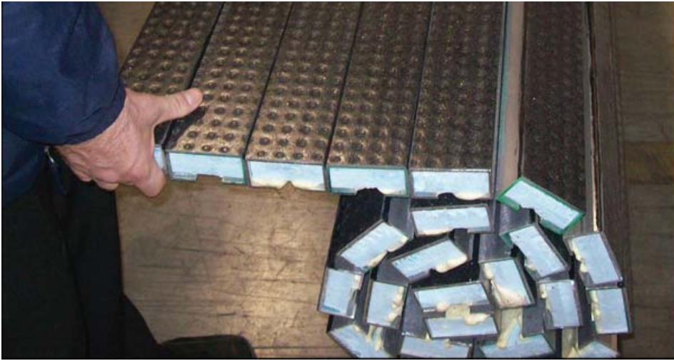
The rolling floor that allows OEM's new CIMS trailer to serve as a functional workspace at any width is just one of the special features that helps this new vehicle serve the ever-changing needs of New York City.
