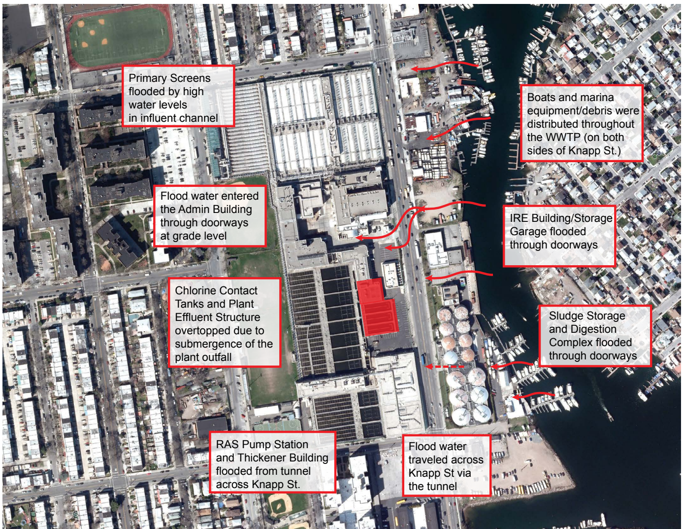
Flood pathways and areas flooded during Hurricane Sandy are highlighted in red.
