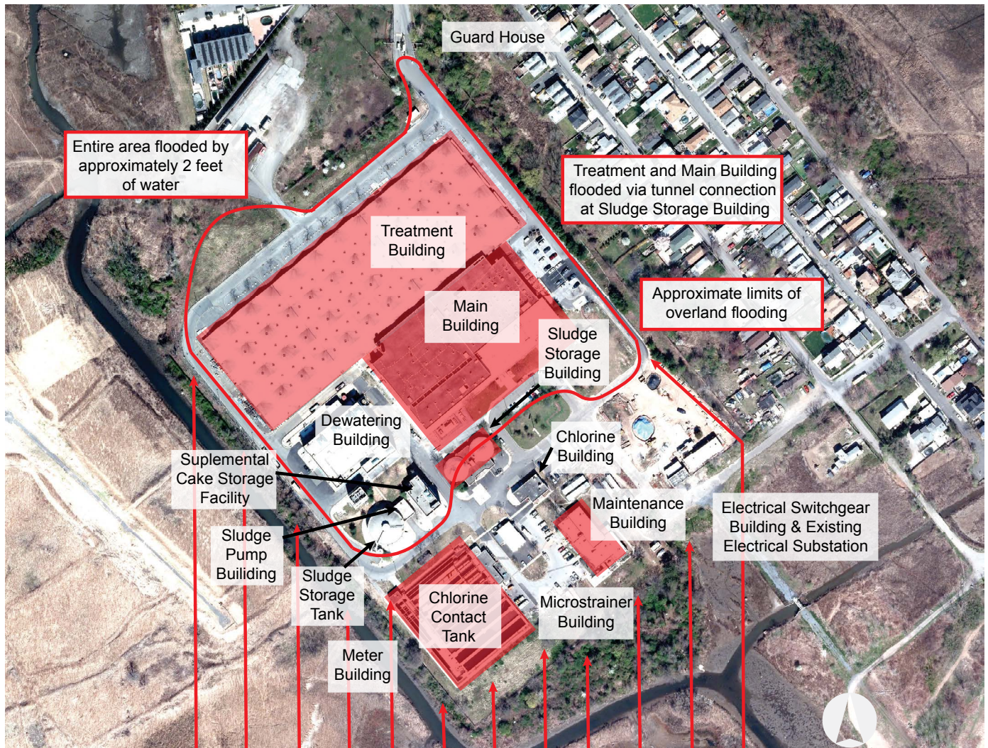
Flood pathways and areas flooded during Hurricane Sandy are highlighted in red.
