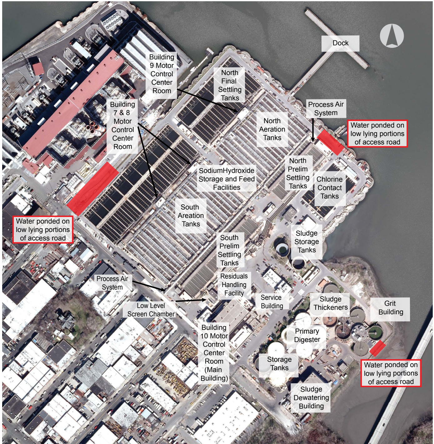
Flood pathways and areas flooded during Hurricane Sandy are highlighted in red.
