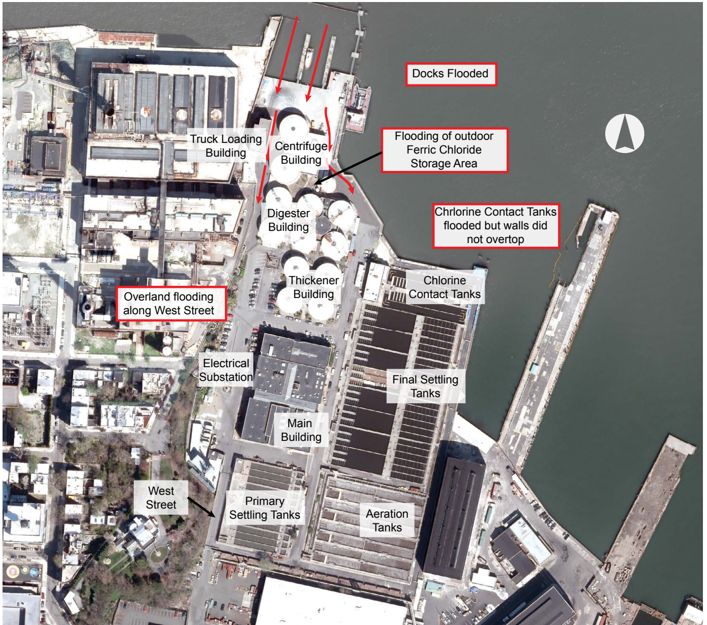
Flood pathways and areas flooded during Hurricane Sandy are highlighted in red.
