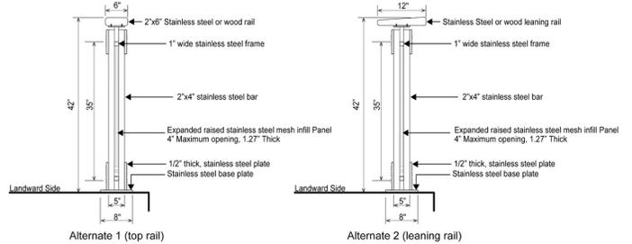
All guardrail components and hardware shall be in unpainted stainless steel and shall conform to any additional standards set forth by DPR.
