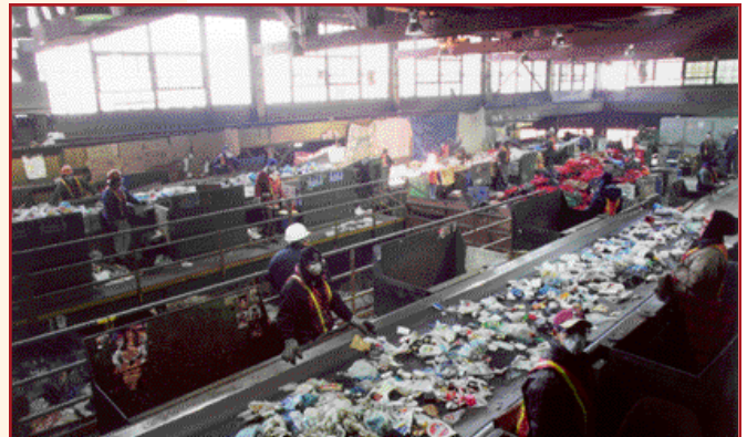
At a material recovery facility (MRF), employees separate plastics from metal and glass on the “sort line.”
