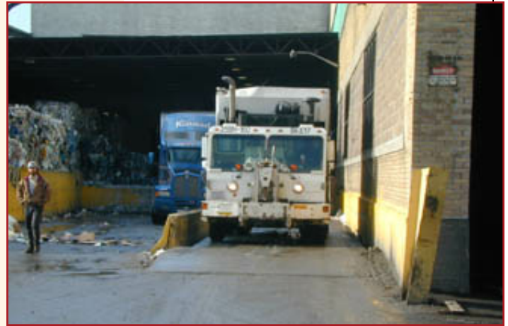
A DOS truck is weighed on a scale before and after tipping its recyclables or refuse load. The data is fed into a computer and tracked daily.
