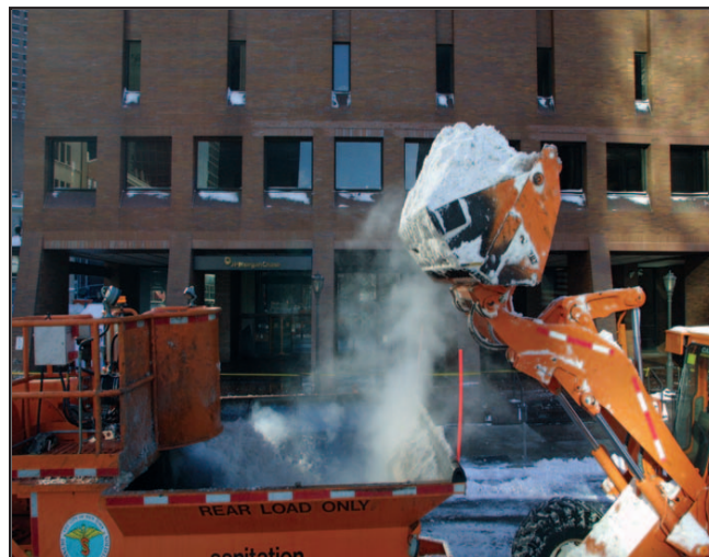
Front-End Loader dumps snow into Snow Melter
