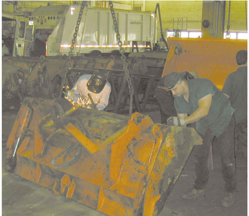
Bureau of Motor Equipment(BME) personnel repair a Front End Loader bucket.
