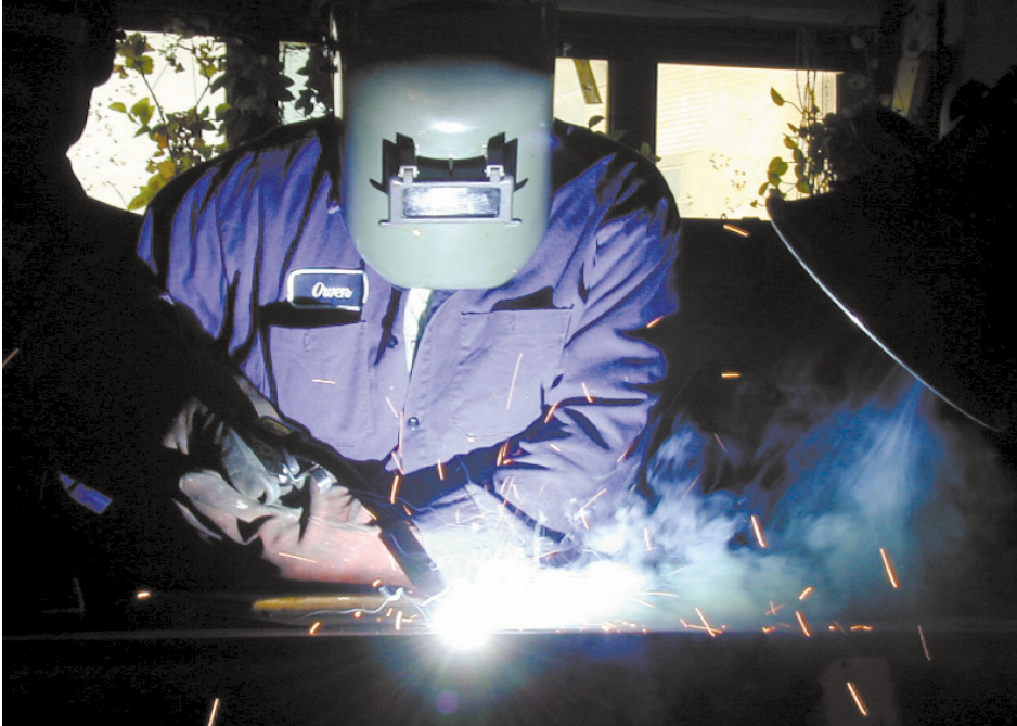
Bureau of Motor Equipment welder repairs plow equipment.
