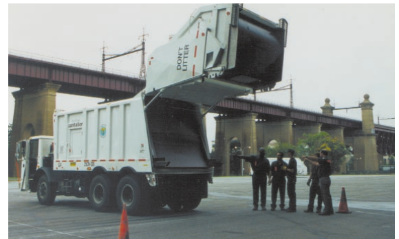
Sanitation Workers learn how to eject contents of collection truck.
