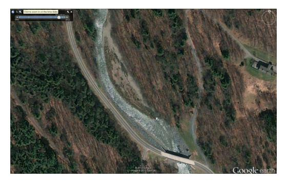
Prior to construction of demonstration project, stream channel threatening embankment, no riparian buffer.
