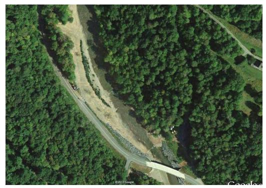
Immediately following substantial completion, buffer bench established, but not yet vegetated.
