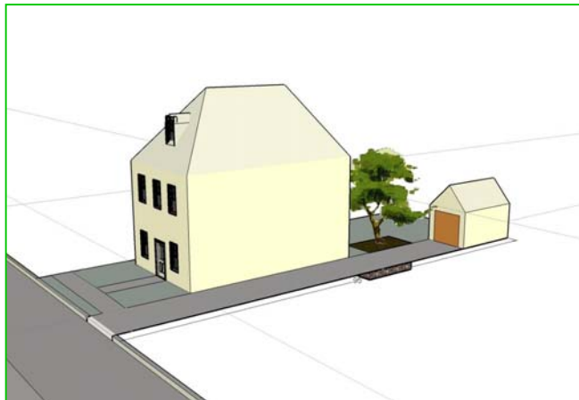
FIGURE 5.2. High Capture for Existing Development: Single Family Residential Prototype w/Tree & Bioinfiltration, 120 sf. Source: Biohabitats, Inc.
