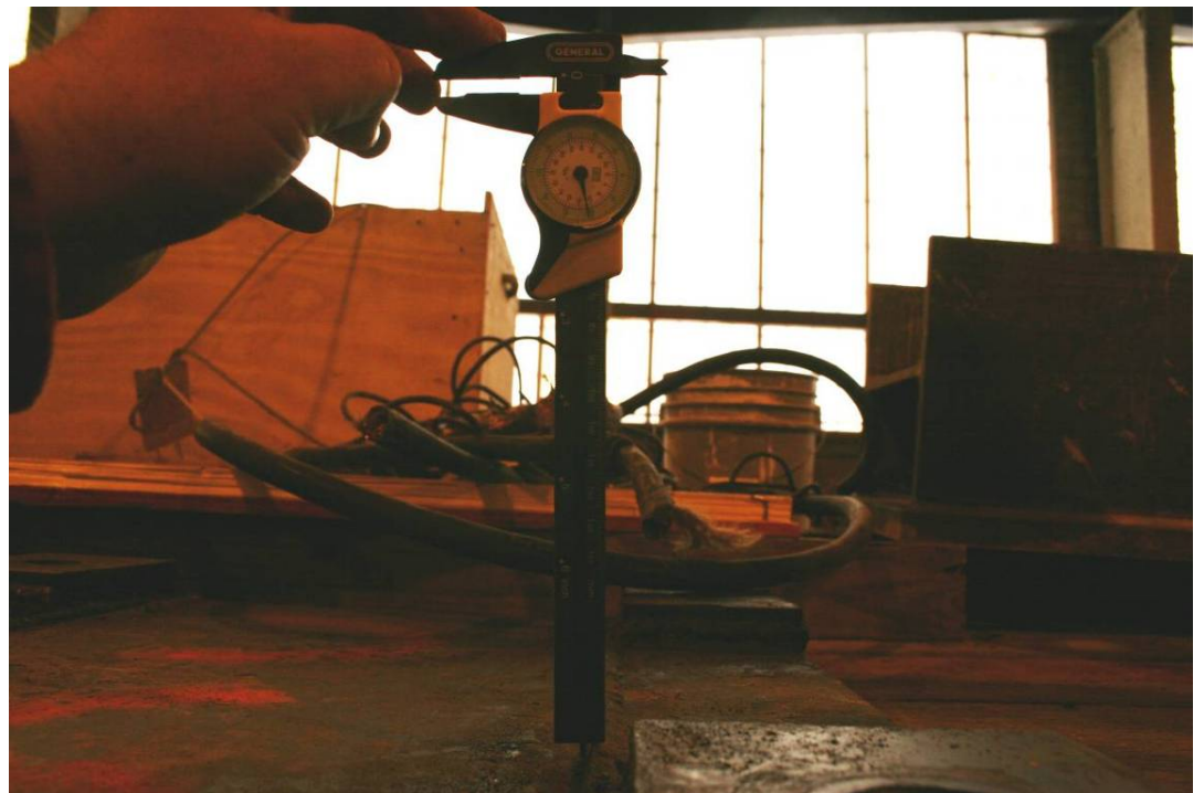
Photograph 3.23 - Fillet weld measurement of base plate 9C. Measurement is shown to be 5 mm, just over 3/16 inch, which is 37.0% under the specified 5/16 inch. Photo by Arup.
