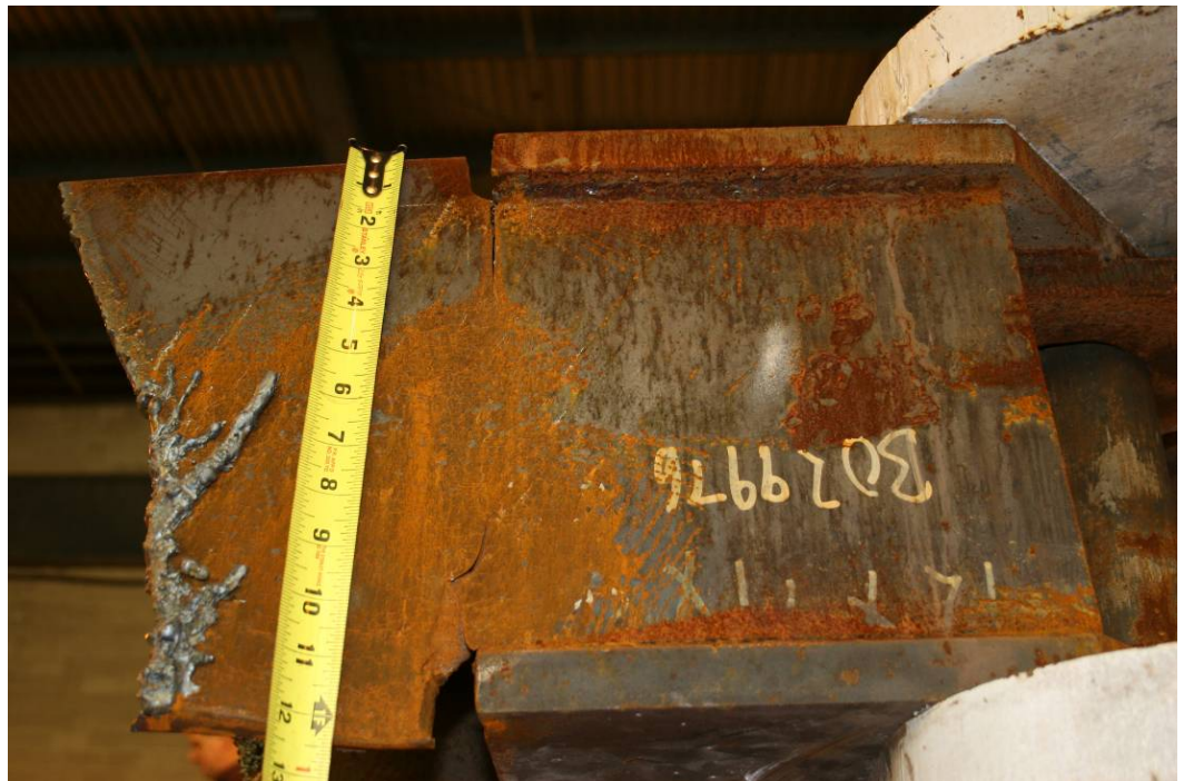
Photograph 1.15 - Fracture of a tie-beam which did not fully fail on the 3rd floor collar. (The fracture of interest is to the right of the tape measure. The damage to the left of the tape measure is a flame-cut (post failure) to assist in the removal of the debris. Photo by Arup.
