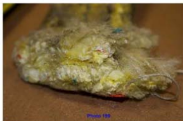
Figure 9. Fracture surface of sling piece 11.
