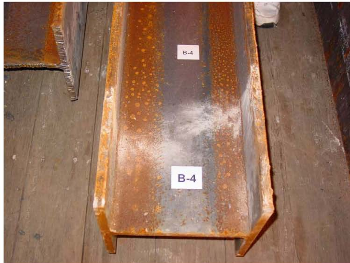
Figure 3 Ninth Floor Horizontal Tie Beam B4 End With Weld Fractures. (Welded to Base Plate 9A).
