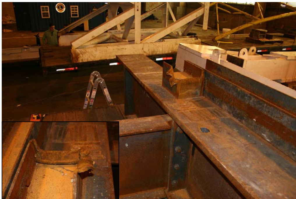
Photograph 7.1 - Dunnage foundation. The inward deformation visible in the closeup of the deformed pocket indicates that the steel plate at the end of the pocket was squashed due to a downward force from the tower legs. Had failure occurred due to a horizontal sliding load the plate would have been deformed in the opposing direction. Photo by Arup.
