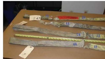
Figure 2. Recovered pieces of slings involved in the crash.
