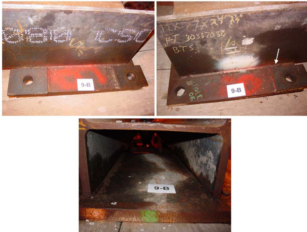
Figure 20 General Views of the Base Plate/Tie Beam Welds From Base Plate 9B.(Arrow Shows Location of Weld Toe Crack)
