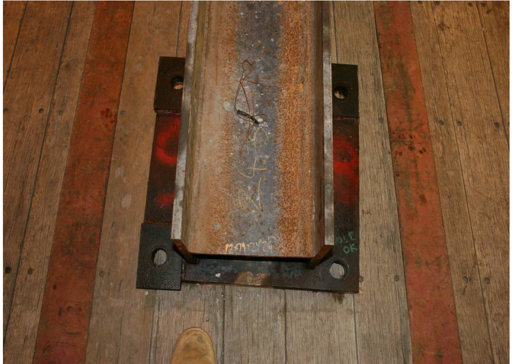
Photograph 9.3 – Base plate 9B from floor level 9. The tie-beam is still attached. Photo by Arup.
