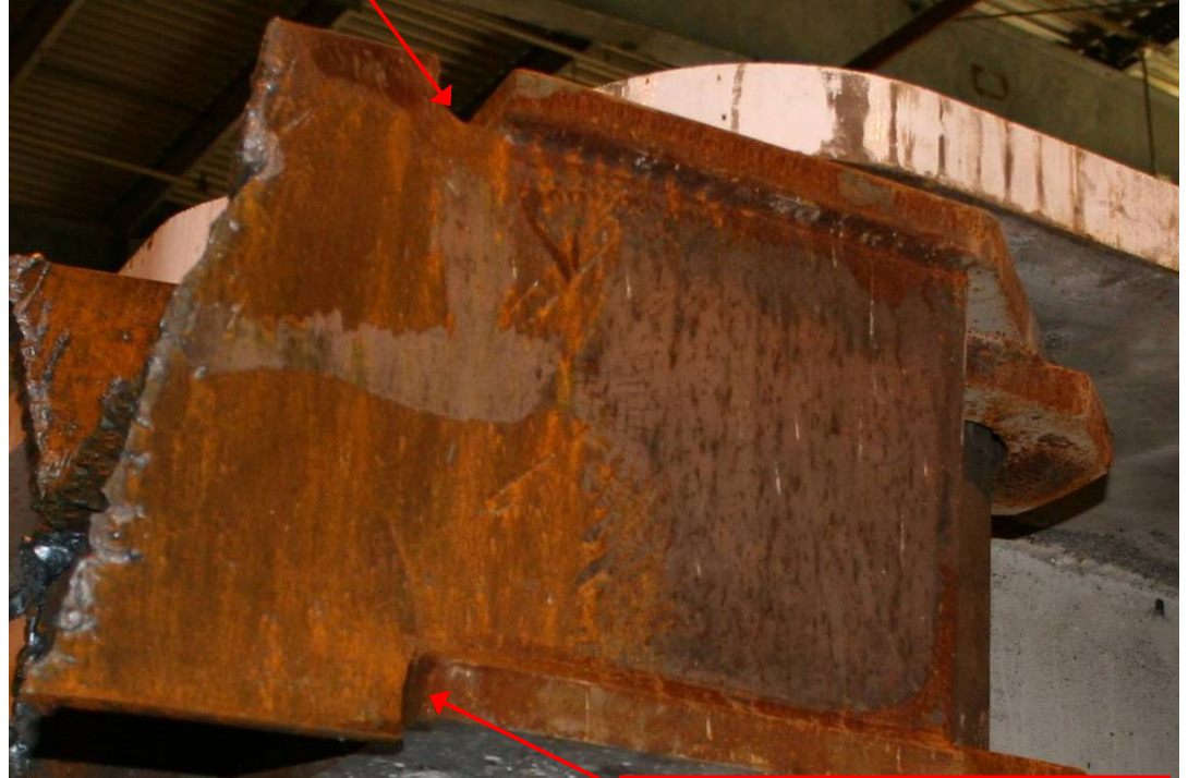
Photograph 3.21 - Tie-Beam from the 3rd floor level. Collar end. Note the lack of clearance between the end of the failed fillet weld and the radiused cut in the beam flange as well as the excessive cut for the bottom plate. The top plate appears to have been fabricated as specified. Photo by Arup.
