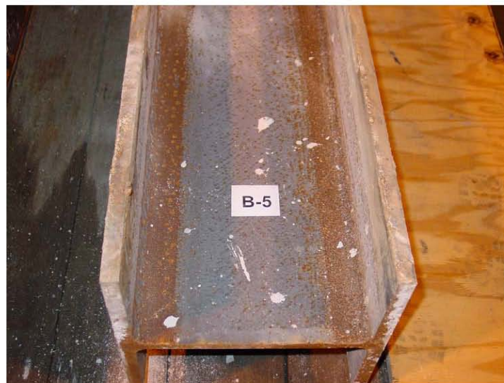
Figure 4 Ninth Floor Horizontal Tie Beam (B5) End With Weld Fractures. (Welded to Base Plate 9C).
