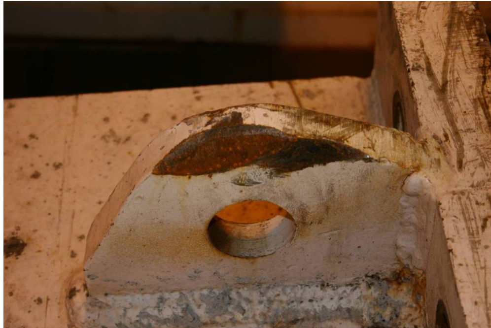
Photograph 3.12 - Collar C2-A chain block attachment point. Note the unprotected edges on which the wire rope sling would have been bearing (typical for all chain block and lifting attachments for all collars).. Photo by Arup.
