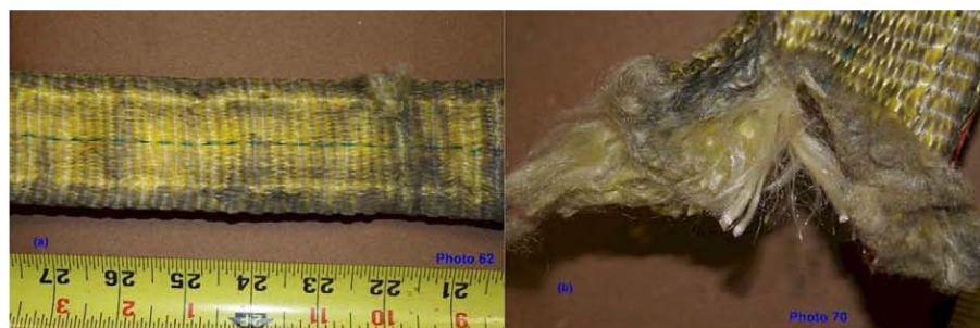
Figure 5. (a) Sign of stress on sling piece 2A, (b) Fracture surface of sling piece 2A
