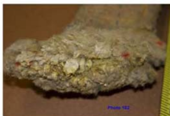
Figure 7. Fracture surface of sling piece 4A.
