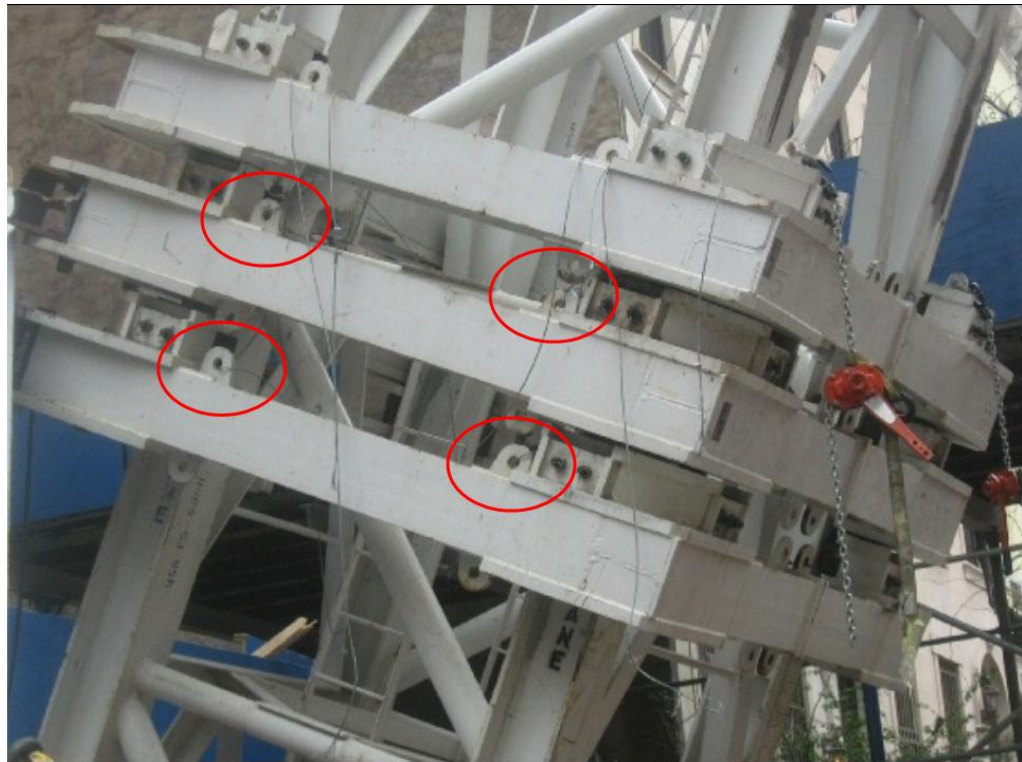
Photograph 3.5 - View of the west elevation of the collapsed tower collars. The location of visible wire rope attachments to the collars are circled. Note the lack of thimbles in the formed sling. Photo from New York County District Attorney 328_58.jpg.
