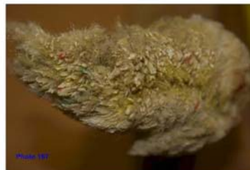
Figure 8. Fracture surface of sling piece 7A.
