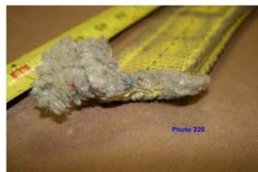
Figure 10. Fracture surface of sling piece 12.
