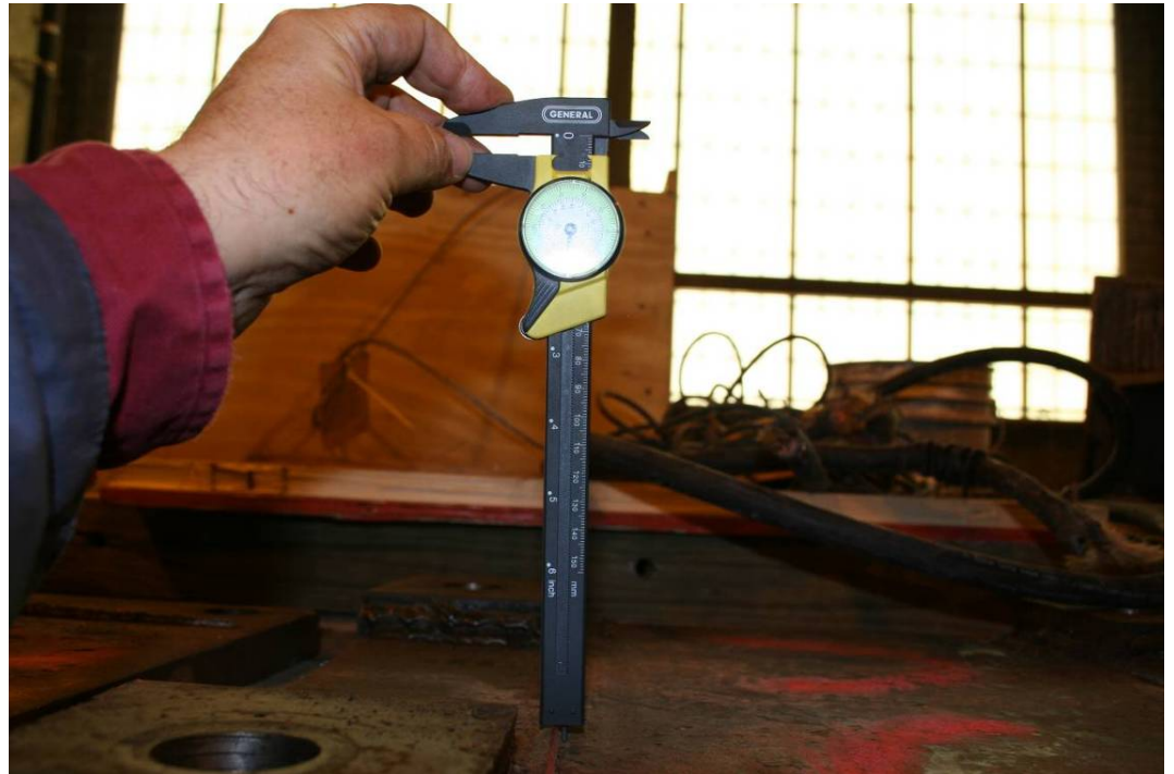
Photograph 3.22 - Fillet weld measurement of base plate 9C. Measurement is shown to be 7 mm, just under 9/32 inch which is 11.8% under the specified 5/16 inch. Photo by Arup.
