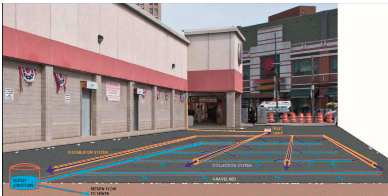
Figure 14: Potential Gravel Bed to Control Runoff from New Development
