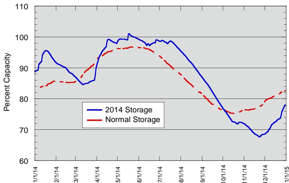
Figure 2.8 2014 Systemwide usable storage compared to normal storage. Storage greater than 100% is possible when the reservoirs are spilling or when the water surface elevation is greater than the spillway elevation.
