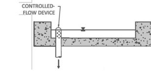
Detention tank – enclosed tank with a device that controls the release rate of water. Common devices include a controlled-flow orifice or pump.
