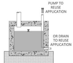
Cistern – container that is used to store runoff below grade. Typically connected to a system that will automatically and continuously reuse water over time.
