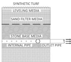
**Porous pavement** - pavements that contain voids which allow runoff to percolate into underlying layers. The surface of these systems can either be entirely porous pavement or a grid of pavers and porous materials, such as grass or gravel. Common underlying layers include a leveling course, sand filter media, and a stone base.
