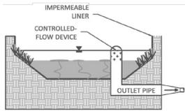
Wet basins/ponds – a permanent pool of water used to treat stormwater, usually underlain by impervious soils or a liner. These systems allow for additional, temporary storage above the permanent pool.
