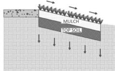
Vegetated swale – open, shallow channels with short vegetation along bottom and sides that infiltrates water as it is conveyed along swale. Commonly consists of a
