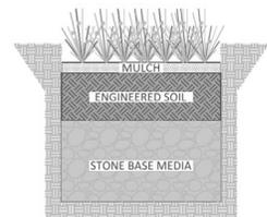
Rain garden – landscaped shallow depression that captures surface runoff. Typically used in residential applications. Similar to bioretention, but components are
