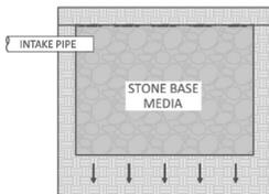
Stormwater gallery – subsurface area (typically rectangular) that is excavated and then filled with stone base, prefabricated structures, chambers, or pipes used to store water. Usually larger than a typical dry well system and, as a result, may treat larger drainage areas.
