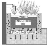
Tree planting (or preservation) – standalone trees (planted or preserved) that capture surface runoff. Commonly consists of a shallow surface ponding area and topsoil for tree planting. In the case of plantings, may also include a shallow drainage layer. This practice is counted towards a reduction of impervious area when calculating the runoff coefficient, rather than towards a required storage volume.
