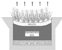
Stormwater planter – self-contained planter box with a concrete bottom. Commonly consists of a surface ponding area, mulch layer, engineered vegetation, and a stone base drainage layer. May also have weep holes to help drain excess water.
