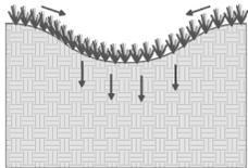
Dry well – subsurface shaft (circular) that is typically excavated or augured and then filled with a stone base or a prefabricated structure used to store water. When the depth of a dry well is greater than its diameter, which is common, an EPA injection well permit may be required (visit epa.gov/iuc for more details).
