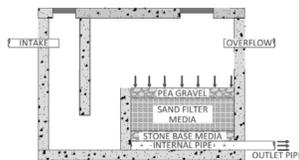
**Organic filter** - typically a prefabricated chamber that contains a filter bed of organic media. The chamber also facilitates the temporary storage of water above the filter bed as it percolates through the organic media filter.
