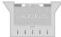
Synthetic turf field – synthetic turf material that allows runoff to percolate into underlying layers. Common underlying layers include a shock absorbing pad, leveling course, and a stone base. Due to their size, many synthetic turf fields also include internal pipes to help spread water evenly across the entire storage area.
