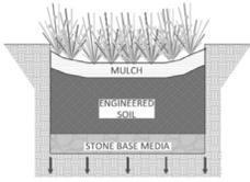
Stormwater planter – self-contained planter box with a permeable bottom. Commonly consists of a surface ponding area, mulch layer, engineered soil with vegetation, and stone base.
