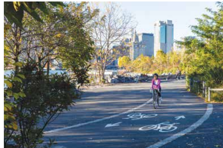
◀ Bike stamps and a cobblestone strip delineate a two-way bicycle path from pedestrian lanes and waterfront seating areas.
