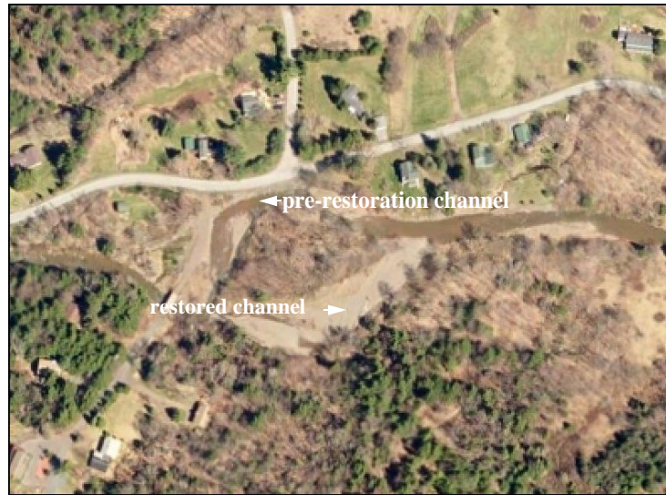
Figure 4.21 East Kill at Vista Ridge prior to restoration. The East Kill had shifted to flow primarily through a side channel that ran alongside Colgate Lake and Vista Ridge Roads, leaving the primary channel, historically aligned with the bridge, nearly dry.
