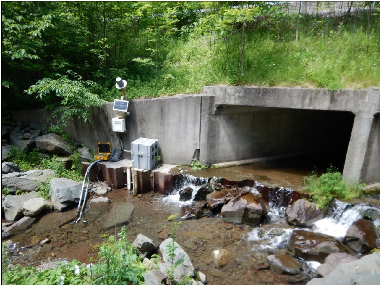
Figure 3. Primary water quality monitoring station 01362322 for Myrtle Brook in the Stony Clove watershed. Primary stations monitor stream discharge and turbidity at 15-minute intervals and use automated and manual sampling for suspended-sediment concentration across a range of discharge conditions.
