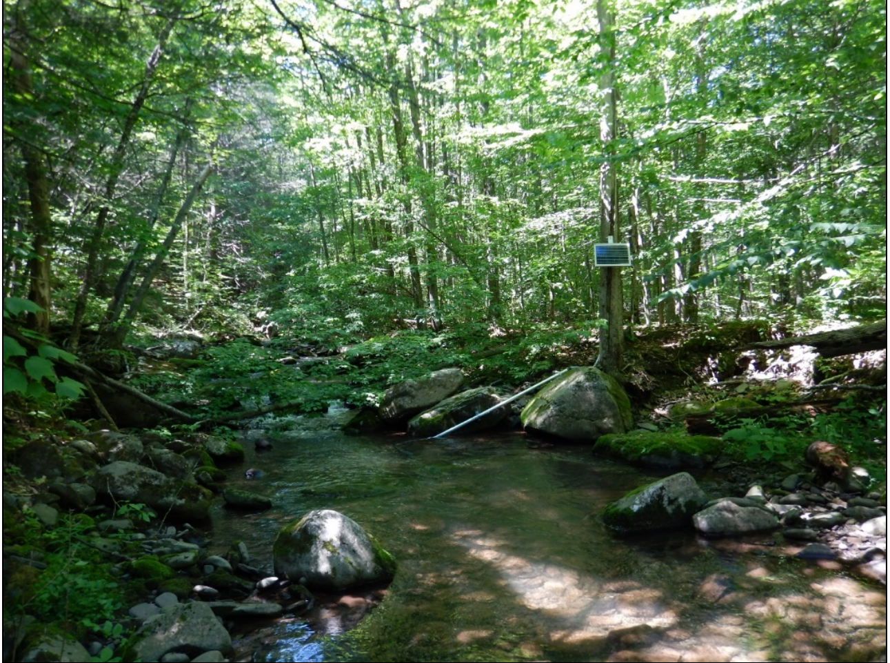
Figure 4. Secondary water quality monitoring station 01362365 on Ox Clove Creek in the Stony Clove watershed. Secondary sites monitor turbidity at 15-minute intervals.
