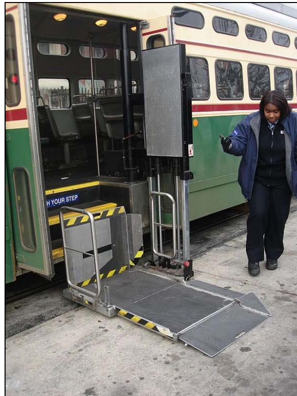
Figure 4-13: PCC Wheelchair Lift
