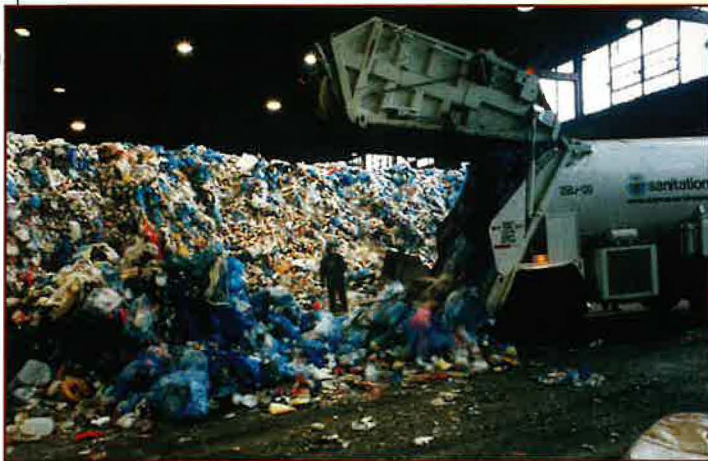
DOS workers tip blue bags full of metal, glass, and plastic recyclables at a material recovery facility (MRF) for processing by private contractors.
