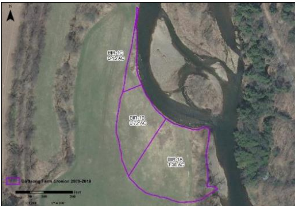
Figure 8. Orthoimagery of Birdsong Farm on the West Branch Delaware River with superimposed extents of streambank erosion as of 2019.
