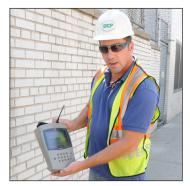
If a pipe breaks in the distribution system and no one is around to hear it, does it make a sound? Just ask **John Lobello**. John—one of four supervisors in the Leak Detection Unit in the Bureau of Water and Sewer Operations—and his team use sound monitoring equipment to listen to our water as it flows through mains on its way to being distributed throughout the city.
