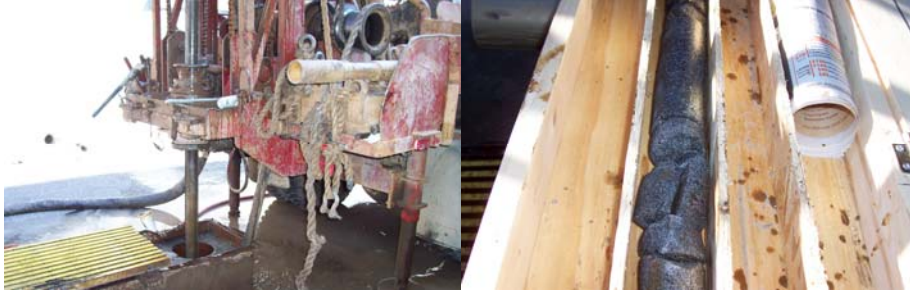
Conducting Soil Borings in November 2008 as Part of the Seismic Retrofit Design of the Manhattan Bridge. Drilling to a Depth of Approximately 210 Feet to Obtain an 8-foot Long Hard Rock Sample. A 2 1/2 -Foot Long Hard Rock Sample Taken From a Depth of Between 202 and 204 1/2 Feet.
