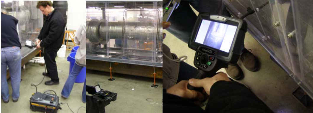
Director of Bridge Management Kevin McAnulty Utilizing a Borescope to Investigate the Suspension Cable Model at Columbia University. The Cable is 20 Inches Thick and 20 Feet Long, Made of 10,000 Steel Wires, Each Five Millimeters in Diameter. Sensors in the Cable Measure Corrosion Rates, Temperature, Humidity, Acidity and Chlorine Content, and Microphones Detect Cracking in the Steel Strands. (Credit: Bojidar Yanev)
