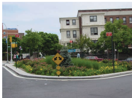
Planted triangle. Shorter plants are located near the edge to maintain sightlines: Macombs Road and Grand Avenue, Bronx (Credit: DPR)
