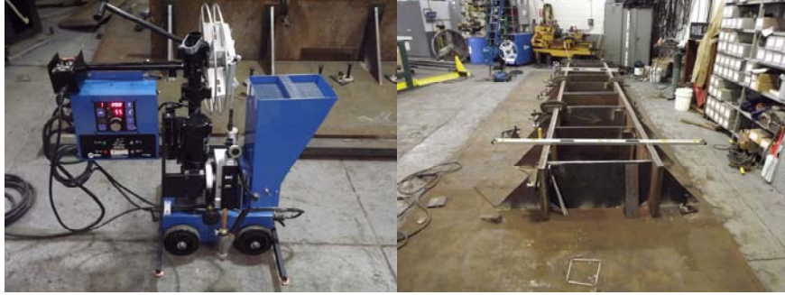
The Sub-Arc Welder Provides a Purer Weld With Less Contaminants From the Atmosphere. The Beam. (Credit: Thomas Whitehouse)
