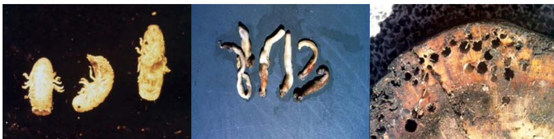
Marine Borer – Limnoria Species. Marine Borer – Teredo Species. Teredo Damage (Holes up to ¼" Diameter).
