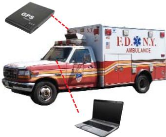
2 Mobile Data Terminal in ambulance sends coordinates by radio: unit location, time of operational status, distance traveled.
