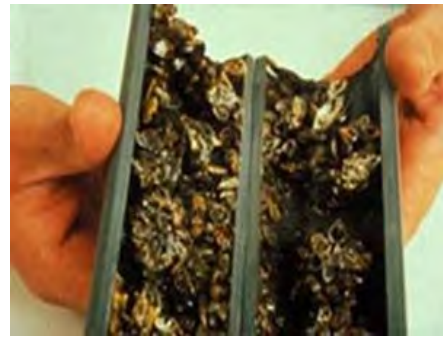
Figure 5.6 Zebra mussels clogging a pipe. http://dnr.wi.gov/org/water/success/2008/bal-last.htm .
