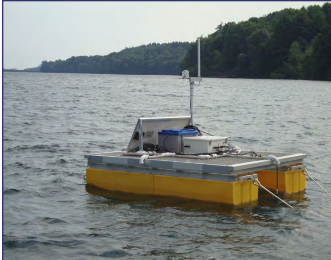
Figure 1.8 Water quality monitoring buoy, part of a robotic network in Kensico Reservoir.
