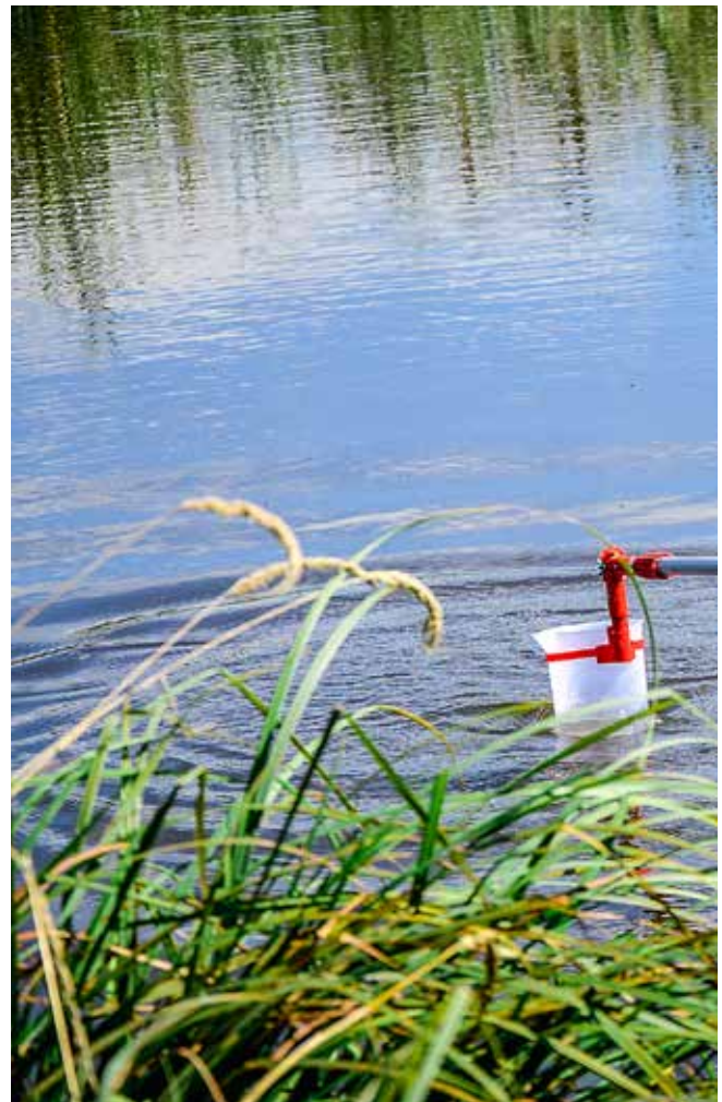
Sampling collection using an extended bucket to prevent contamination
