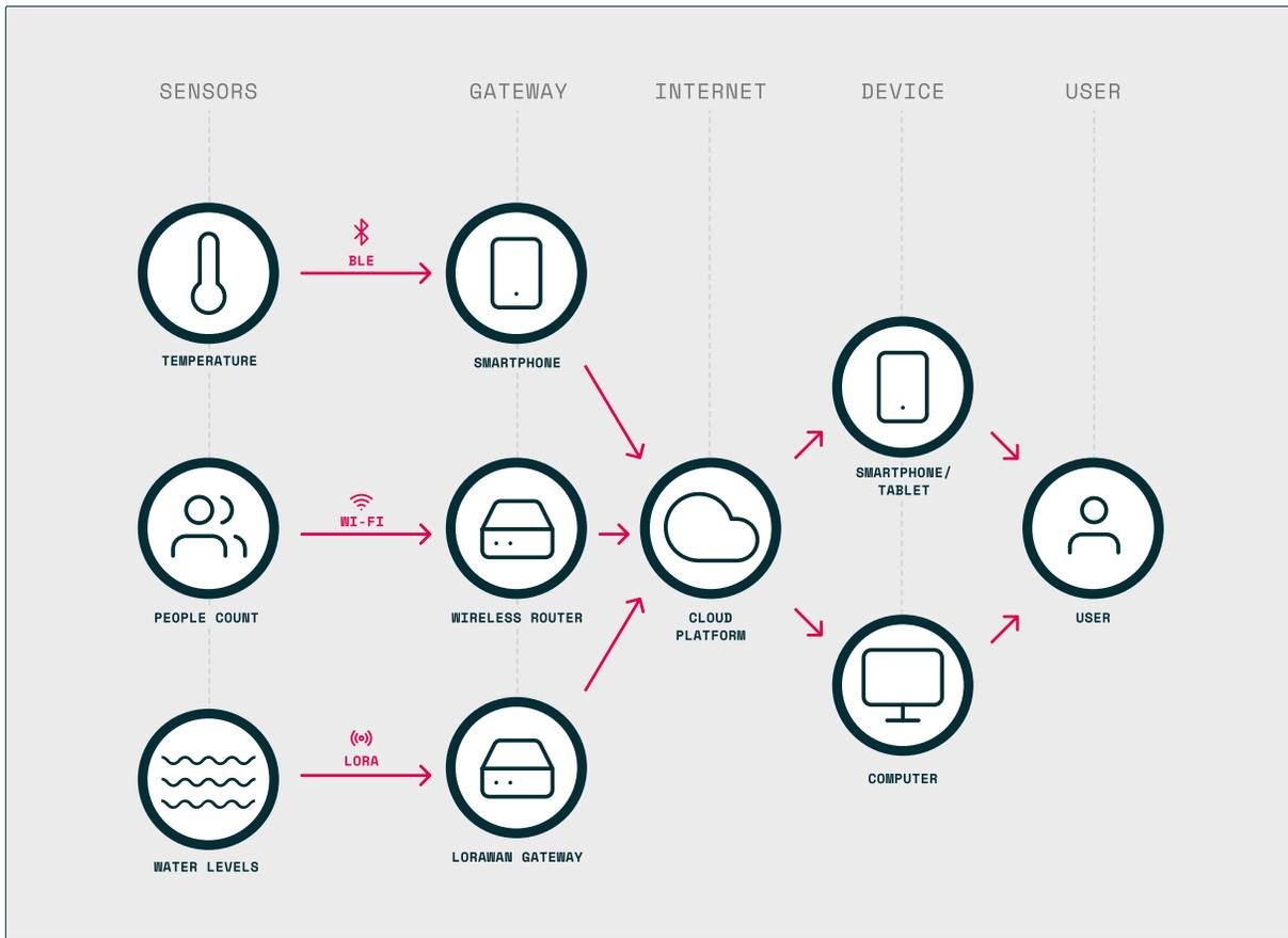
[FIGURE 04 ▲ ] An example of basic IoT system architecture
