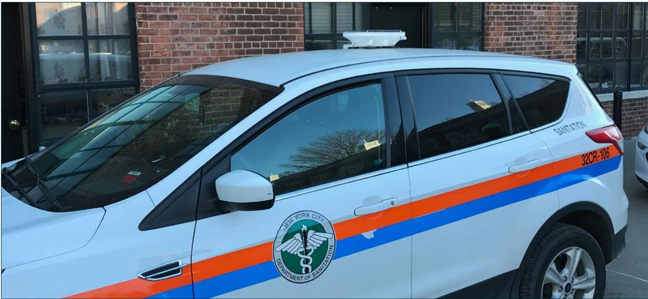
[FIGURE 15 ▲ ] An MIT CityScanner sensor node on top of a New York City Department of Sanitation vehicle.
