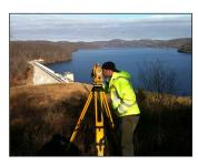
Now: DEP continues conduct land surveys today to locate and maintain boundaries and property lines in order to prevent encroachment, water quality degradation, recreation overuse, and trespass. While still employing a tripod to mount the surveying instrument, modern equipment is elec-
