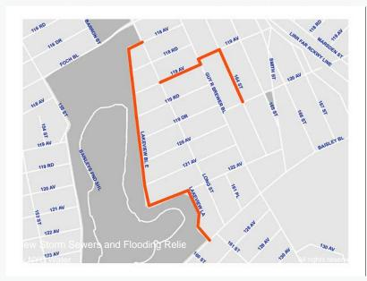
More than 4,700 feet of new storm sewers were installed in the project area, ranging in size from 12 to 42 inches, along with 50 new catch basins to direct stormwater to the new sewers. Over 26,000 square feet of new sidewalk was installed at the edge of the park along with 4,000 feet of new curb. An additional 15,230 square feet of existing sidewalk and 2,350 feet of curb was replaced throughout the area.
