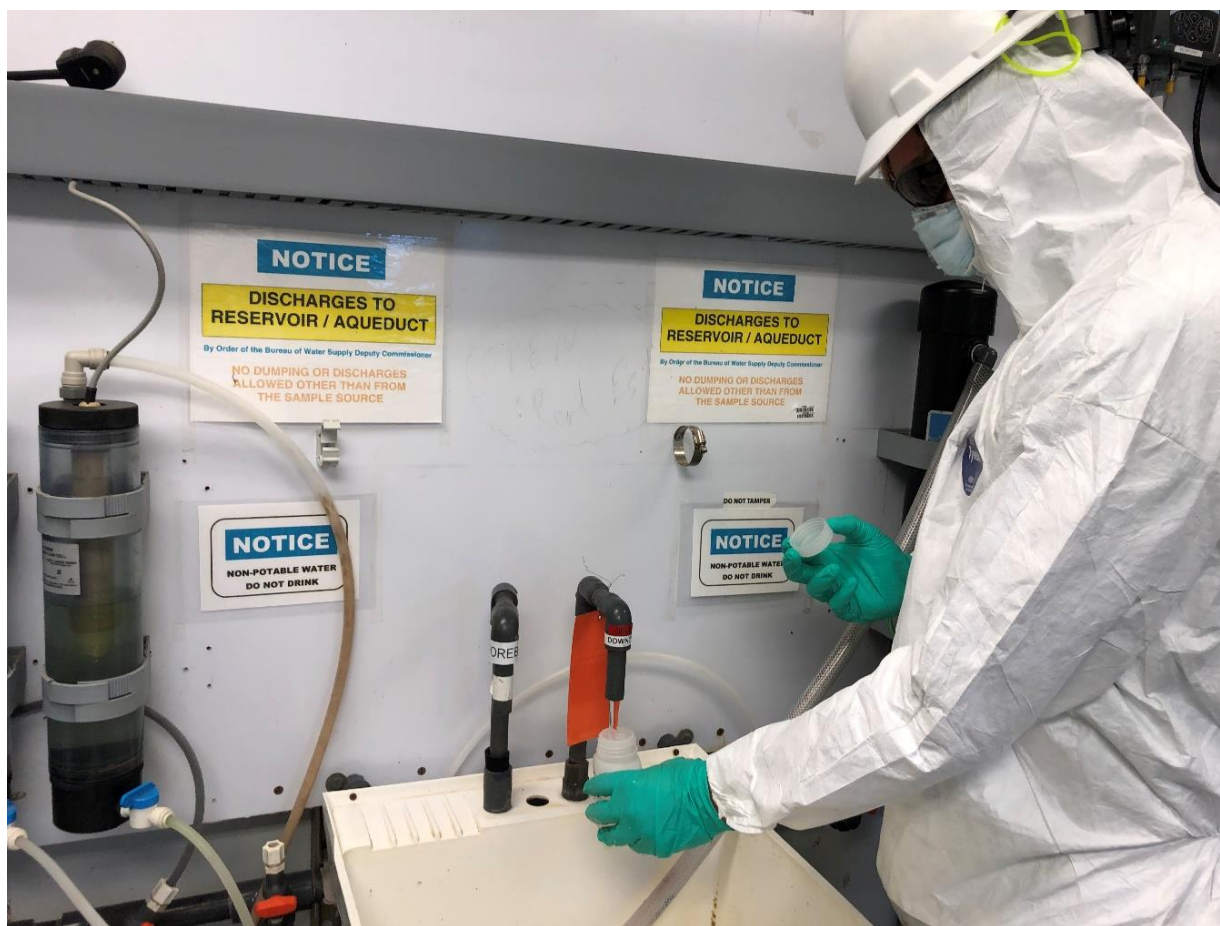
Figure 3. DEP staff sampling for PFAS compounds per instructions from Eurofins-Eaton Analytical LLC.
