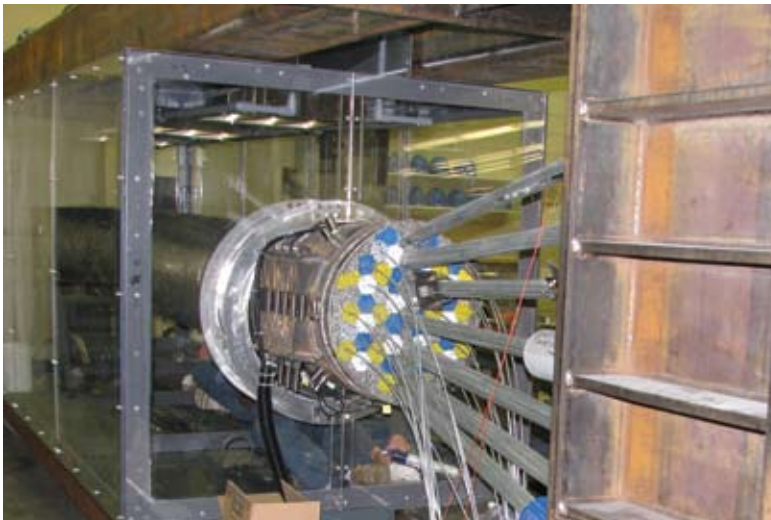
Laboratory testing new technology to monitor the bridge cable corrosion underwater
