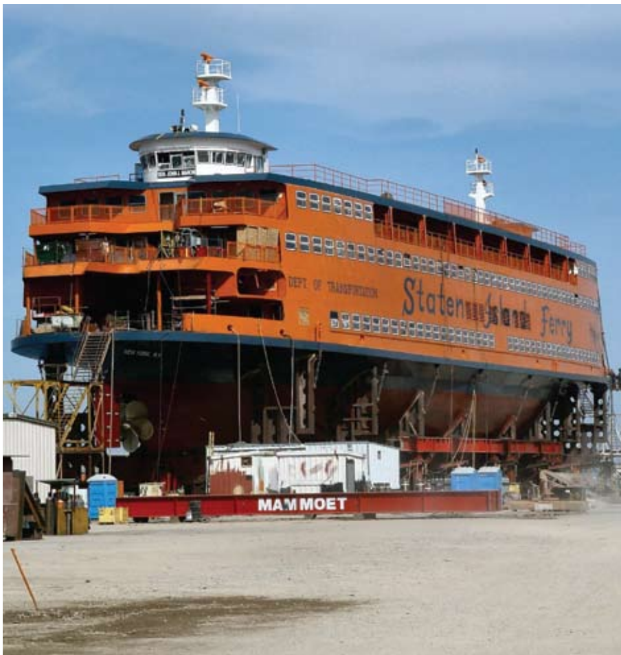
Dry docking during ship construction
