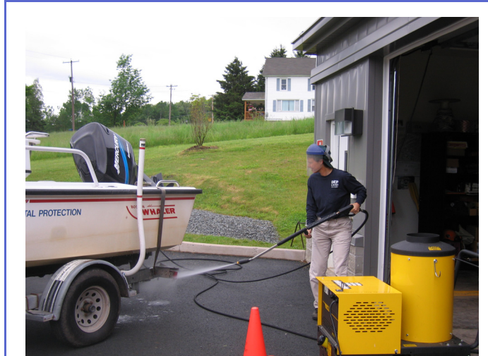
Figure 4.12 Steam cleaning a boat to prevent transport of zebra mussels.
