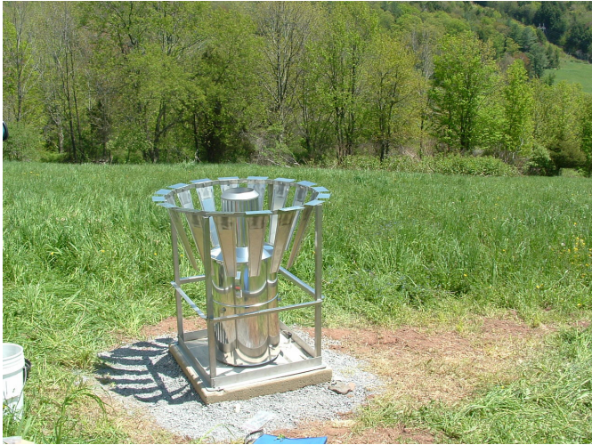
Figure 2.4 An Ott Pluvio precipitation gage located at DEP's Remote Automated Weather Station near Ashland, NY in the Batavia Kill sub-basin of the Schoharie watershed.
