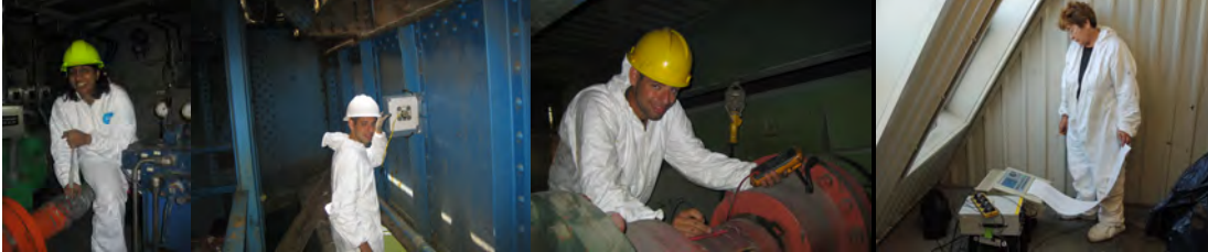
June 2012 - Metropolitan Avenue Bridge. Summer College Intern Nikita Gupta Unsealing the Wire for Strain Gauge Testing. July 2012 - Unionport Bridge. Summer College Intern Kevin Hillery Setting up Inclinator Calibration. August 2012 - Hunters Point Avenue Bridge. Kevin Hillery Checking Strain Gauge Connections With a Millimeter. (Credit: Vera Ovetskaya) August 2015: Assistant Mechanical Engineer Vera Ovetskaya Reviewing the Roosevelt Island Test Results.
