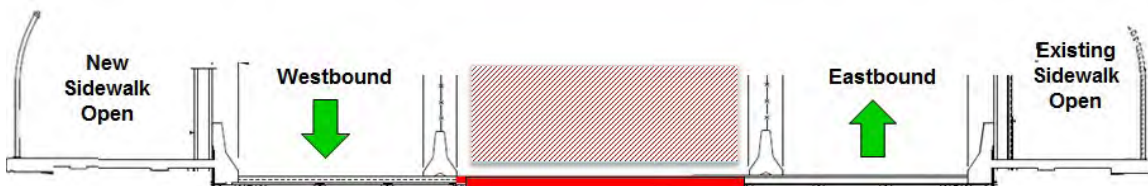
Stage 2 - Center Roadway - 12 Months. The Center Roadway will be Closed. All Traffic Shifts to One Eastbound and One Westbound Lane in Each Direction.
