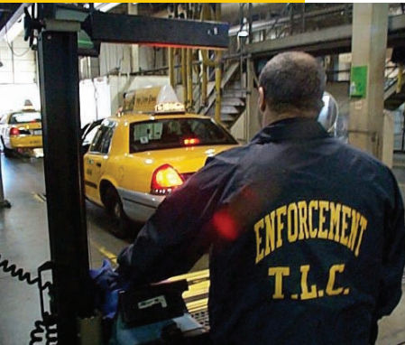
An Inspection Officer performs an emissions test on a NYC taxicab.
