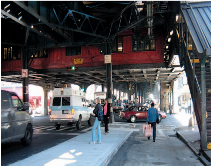
Raised median provides refuge and safety for pedestrians waiting for the bus and crossing the street
