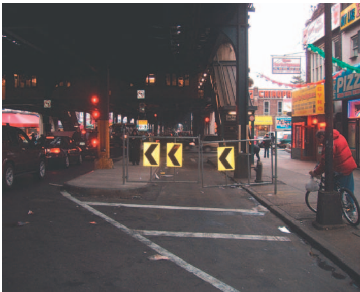
Metal gates, signage and striping direct vehicles to travel lane and protect pedestrian safety
