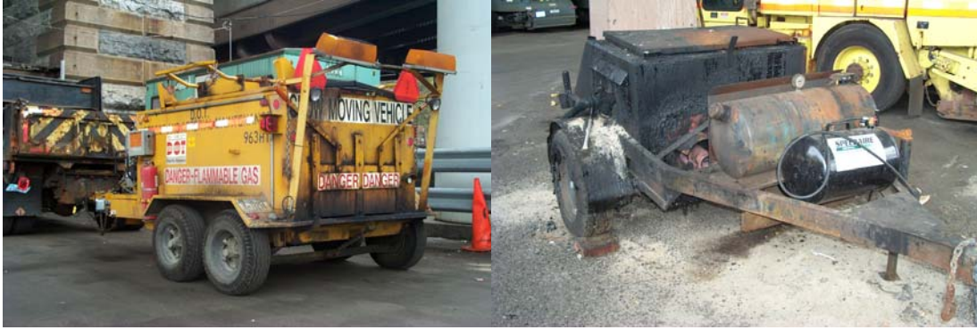
Asphalt Trailer and Tar Kettle. (Credit: Peter Basich)
